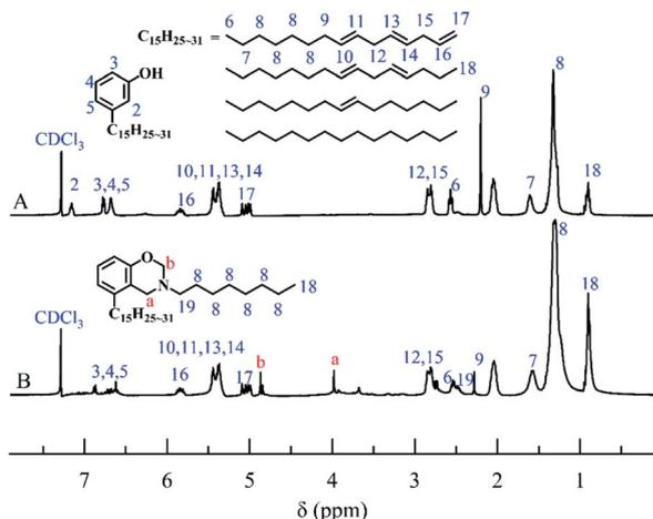
Fig. 2 The  $^1\text{H-NMR}$  spectra of cardanol (A) and CB (B).
