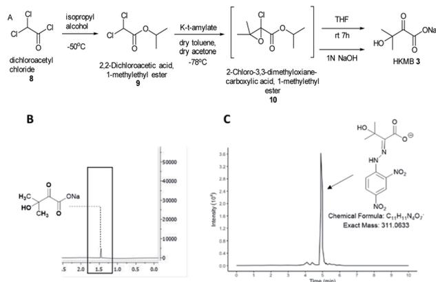
Fig. 2 (A) An optimised synthesis scheme towards HMKB 3 starting from dichloroacetyl chloride 8, via isopropyl 2-chloro-3,3-dimethylloxianoate 10 as a transit intermediate. (B) <sup>1</sup>H-NMR of 3 confirming the presence of the compound. (C) Extracted ion chromatogram (EICs) from LC-MS analysis of 3-DNPH.
