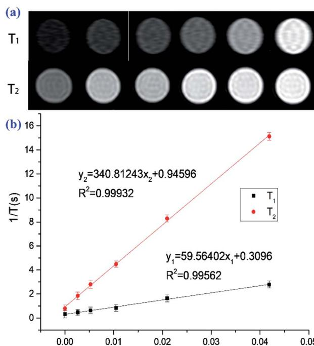
Fig. 3 (a) T1/T2-weighted MR images of PAL@Gd-0.5@PVA composite to pure water (control) at 1.0 T with different concentrations; (b) linear correlation between  $r_1$  ( $T_1^{-1}$ ),  $r_2$  ( $T_2^{-1}$ ) and Gd concentration, based on reading from (a). The  $r_1$  and  $r_2$  relaxivities are the slope of the curve.
