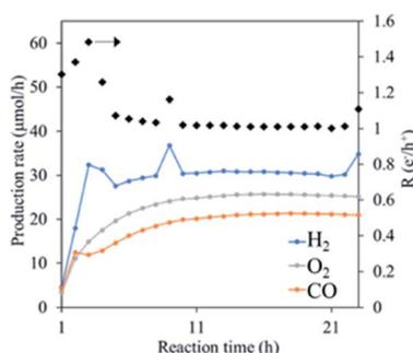
Fig. 3 Time sequences of production rates of H<sub>2</sub>, CO and O<sub>2</sub>, and the electron and hole ratio consumed for the gaseous product formation, R (e<sup>-</sup>/h<sup>+</sup>) under CO<sub>2</sub> reduction tests for sample.
