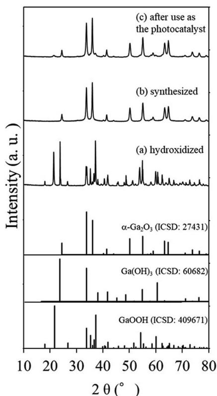
Fig. 1 XRD patterns of the samples (a) hydroxidized (b) synthesized and (c) after use as the photocatalyst. Those for  $\alpha$ -Ga<sub>2</sub>O<sub>3</sub>, Ga(OH)<sub>3</sub> and GaOOH are also given as references.
