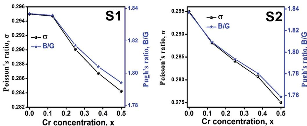
Fig. 15 Poisson's ratio and Pugh's ratio as a function of Cr content for all samples of series S1 ( $\text{Co}_{1-x}\text{Cr}_x\text{Fe}_2\text{O}_4$ ) and S2 ( $\text{Co}_{1+x}\text{Cr}_x\text{Fe}_{2-x}\text{O}_4$ ).
