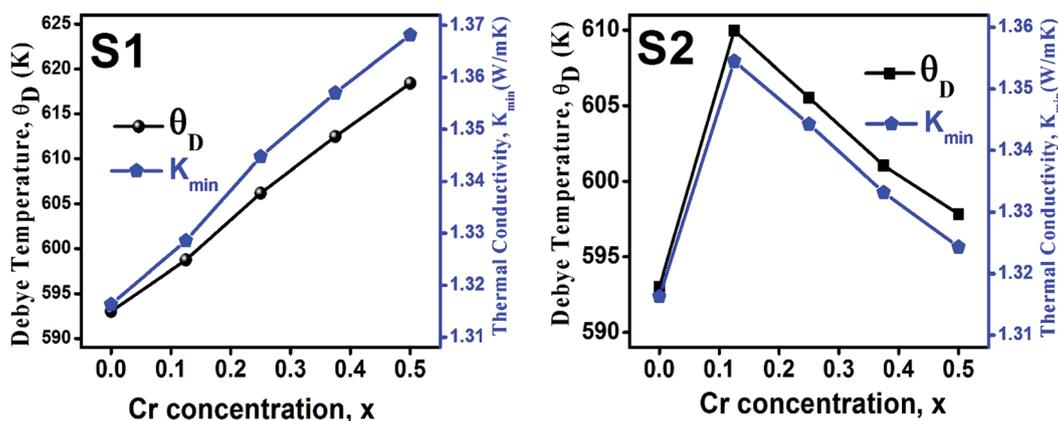
Fig. 16 Debye temperature and thermal conductivity as a function of Cr content for all samples of series S1 ( $\text{Co}_{1-x}\text{Cr}_x\text{Fe}_2\text{O}_4$ ) and S2 ( $\text{Co}_{1+x}\text{Cr}_x\text{Fe}_{2-x}\text{O}_4$ ).
