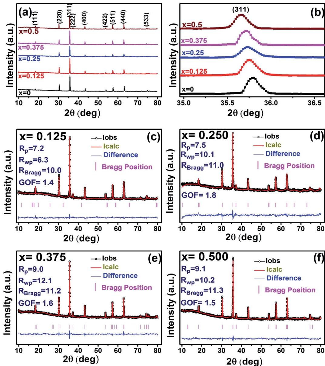
Fig. 3 Rietveld analysis of XRD patterns for all samples of S2 ( $\text{Co}_{1+x}\text{Cr}_x\text{Fe}_{2-x}\text{O}_4$ ) series.
