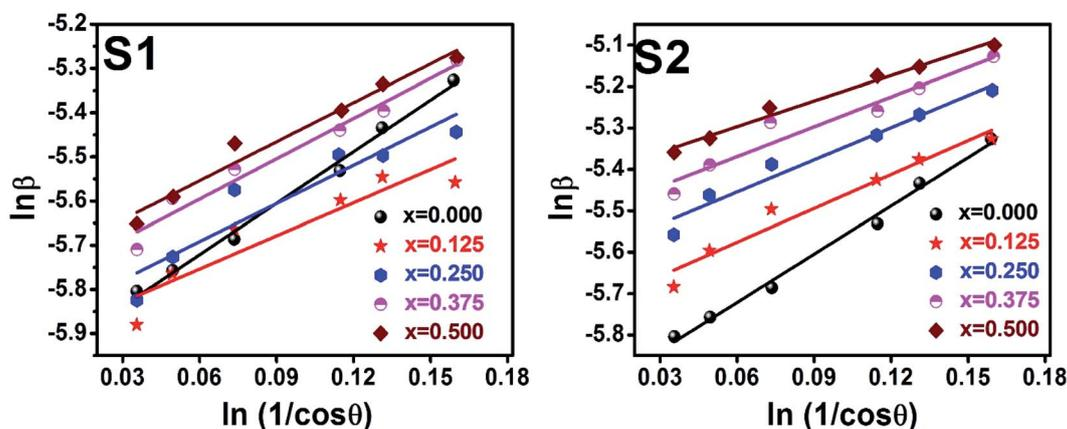
Fig. 8 Modified Scherer plots for all samples of series S1 ( $\text{Co}_{1-x}\text{Cr}_x\text{Fe}_2\text{O}_4$ ) and S2 ( $\text{Co}_{1+x}\text{Cr}_x\text{Fe}_{2-x}\text{O}_4$ ).
