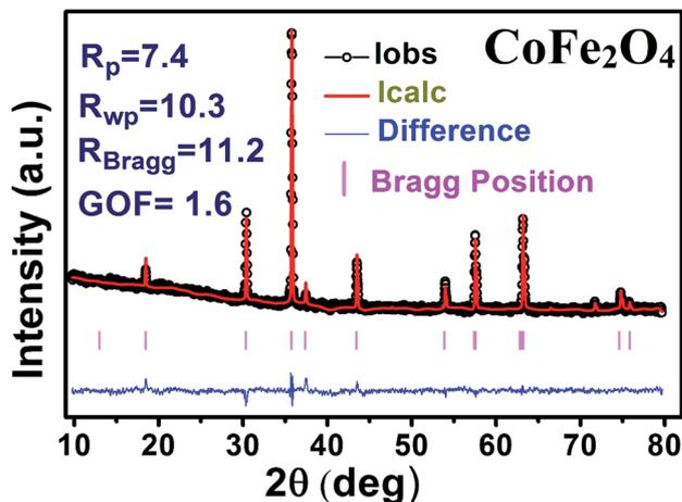
Fig. 1 Rietveld analysis of XRD pattern of CoFe<sub>2</sub>O<sub>4</sub>.
