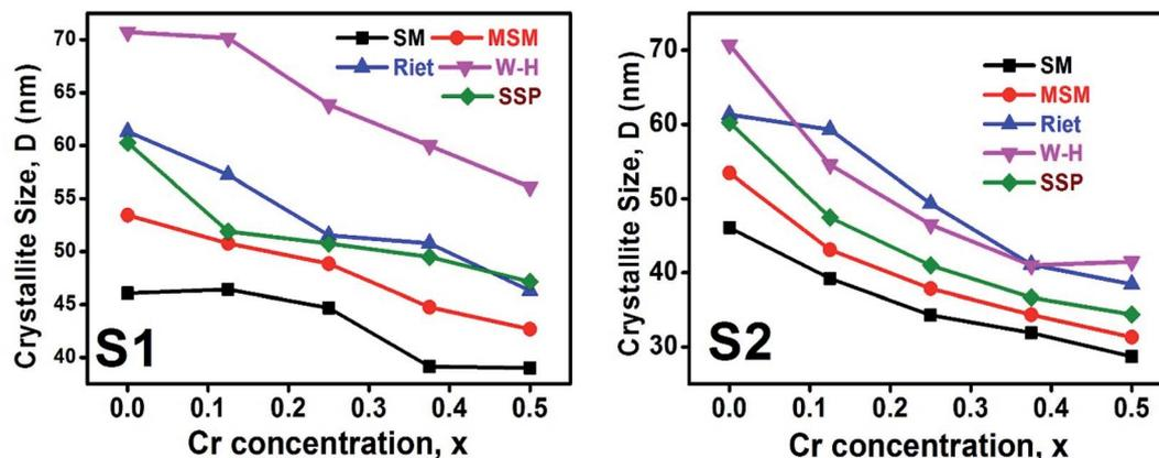
Fig. 11 The  $D$  values calculated using Scherer method (SM), modified Scherer method (MSM), Rietveld method (riet), Williamson–Hall (W–H), and size strain plot (SSP) for all samples of series S1 ( $\text{Co}_{1-x}\text{Cr}_x\text{Fe}_2\text{O}_4$ ) and S2 ( $\text{Co}_{1+x}\text{Cr}_x\text{Fe}_{2-x}\text{O}_4$ ).
