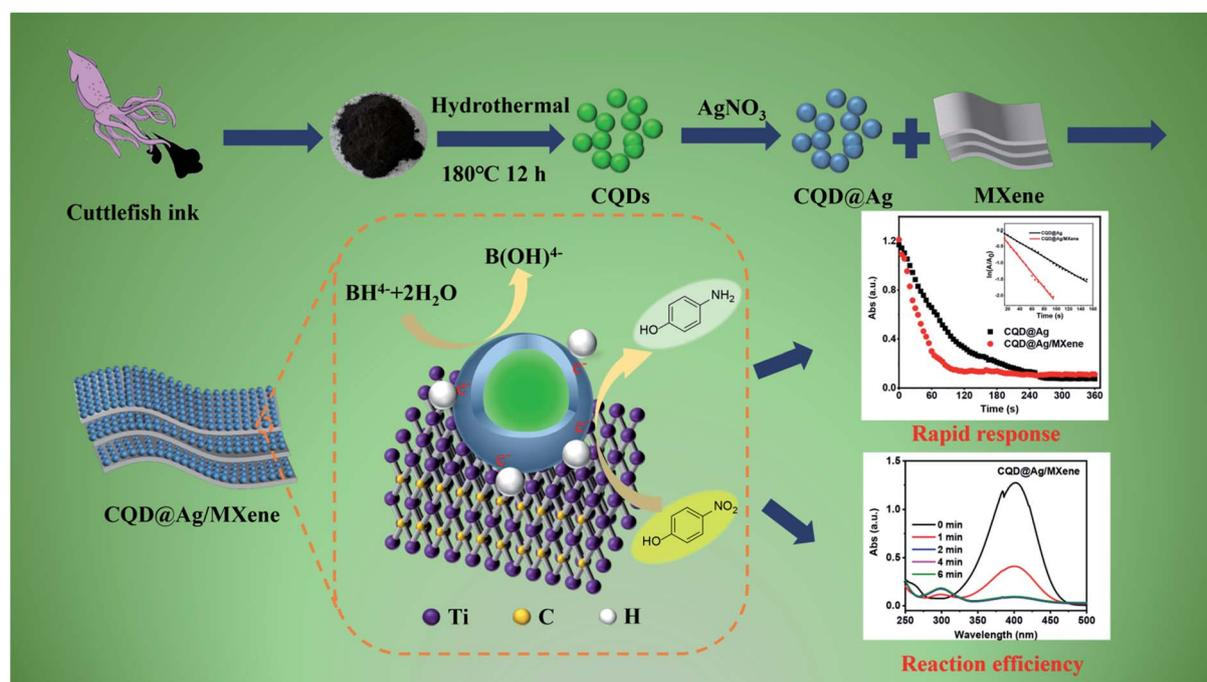
Scheme 1 Schematic illustration of the fabrication of CQD@Ag/MXene and the reduction of PNP in the presence of NaBH<sub>4</sub>.
