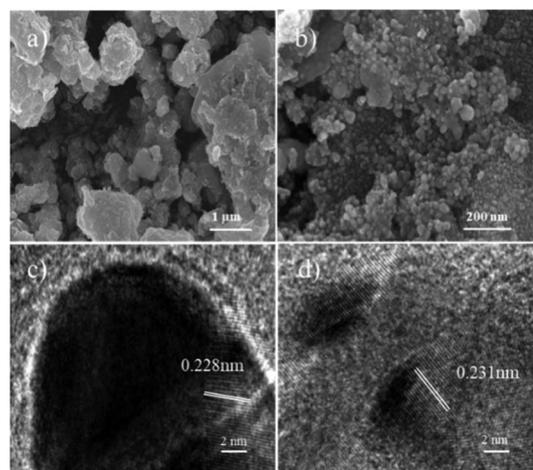
Fig. 1 SEM images of (a) CQD@Ag/MXene and (b) CQD@Ag; HRTEM images of (c) CQD@Ag/MXene and (d) CQD@Ag.
