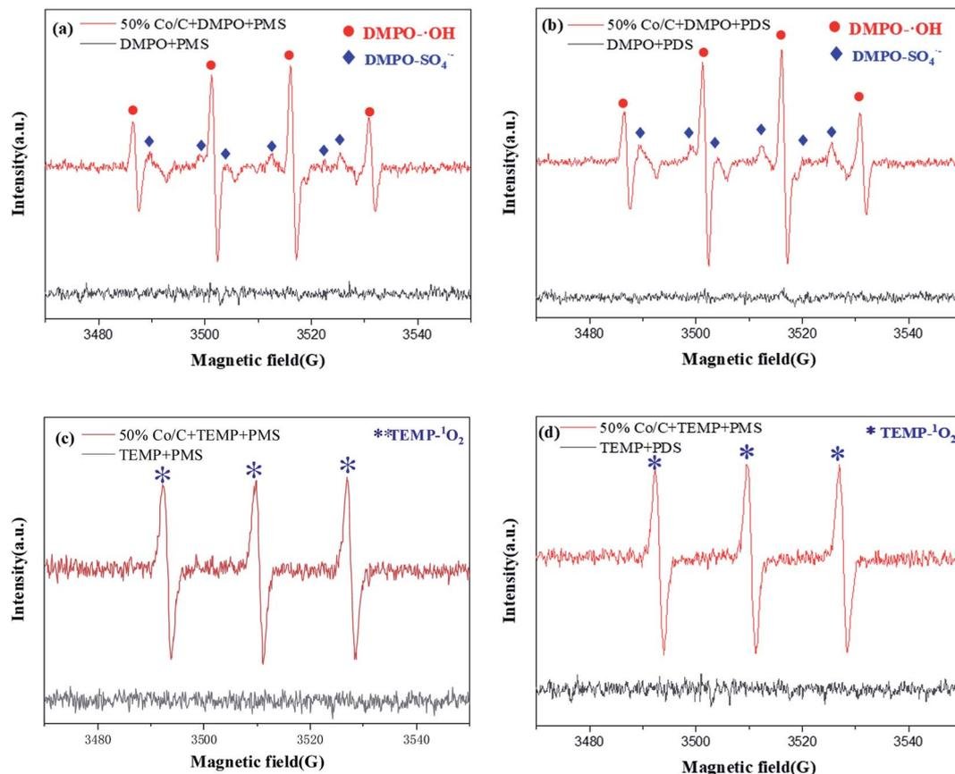
Fig. 9 ESR spectra of PMS and PDS activation by Co/C-50. (a) DMPO- $\cdot$ OH and DMPO-SO $_4^{\cdot-}$  (PMS); (b) DMPO- $\cdot$ OH and SO $_4^{\cdot-}$  (PDS); (c) TEMP- $^1$ O $_2$  (PMS); (d) TEMP- $^1$ O $_2$  (PDS) spin adducts (PMS system:  $m_{\text{catalyst}} = 0.0050$  g, [PMS] =  $0.25$  g L $^{-1}$ ; PDS system:  $m_{\text{catalyst}} = 0.04$  g, [PDS] =  $1.0$  g L $^{-1}$ ).
