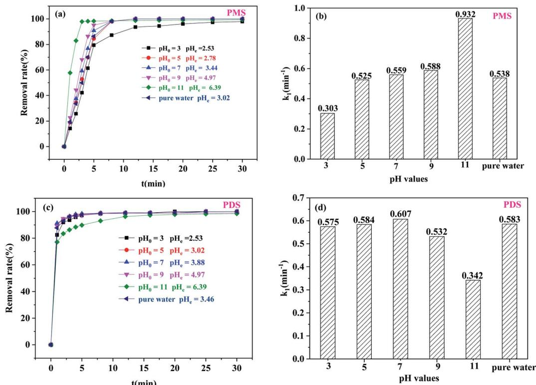
Fig. 7 The effect of solution pH: (a and b) PMS system ( $m_{\text{catalyst}} = 0.0050$  g, [PMS] =  $0.25$  g L<sup>-1</sup>); (c and d) PDS system ( $m_{\text{catalyst}} = 0.04$  g, [PDS] =  $1.0$  g L<sup>-1</sup>) ([BPA] =  $20$  mg L<sup>-1</sup>,  $T = 30$  °C).
