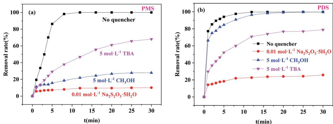
Fig. 8 Free radical annihilation experiment: (a) PMS system ( $m_{\text{catalyst}} = 0.0050$  g, [PMS] =  $0.25$  g L<sup>-1</sup>); (b) PDS system ( $m_{\text{catalyst}} = 0.04$  g, [PDS] =  $1.0$  g L<sup>-1</sup>) ([BPA] =  $20$  mg L<sup>-1</sup>,  $T = 30$  °C).
