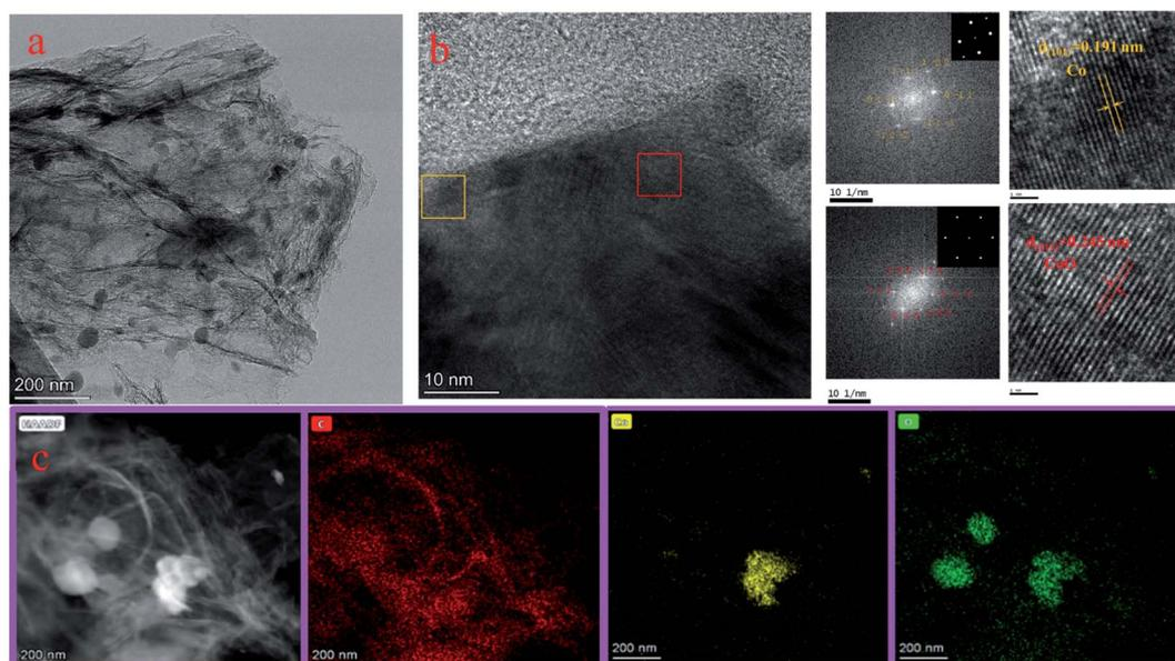
Fig. 3 (a) TEM image, (b) HR-TEM image, and (c) EDS mapping of Co/C-50.
