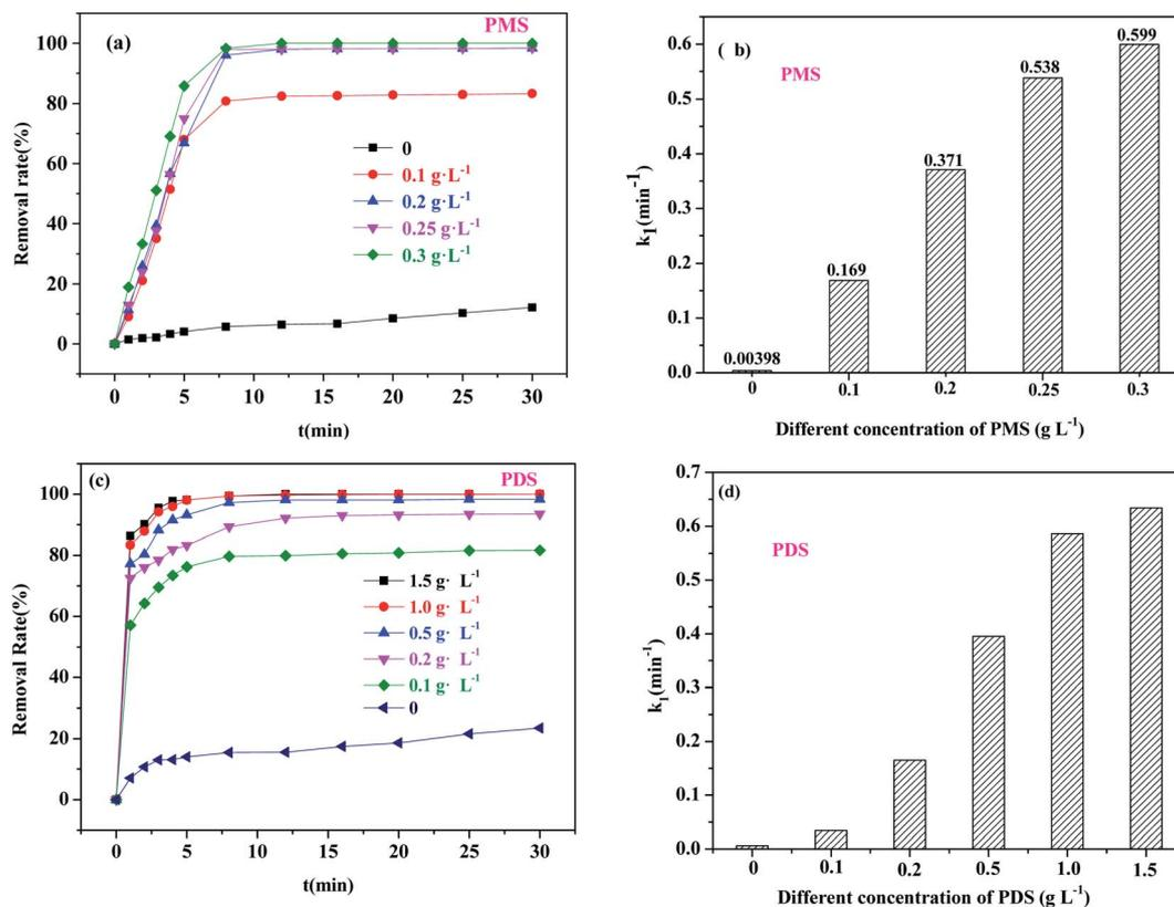
Fig. 6 The effects of PS concentration on BPA degradation: (a and c) BPA degradation as a function of time; (b and d) kinetic constants for BPA degradation (PMS system:  $m_{\text{catalyst}} = 0.0050$  g; PDS system:  $m_{\text{catalyst}} = 0.04$  g,  $[\text{BPA}] = 20$  mg L<sup>-1</sup>,  $T = 30$  °C).
