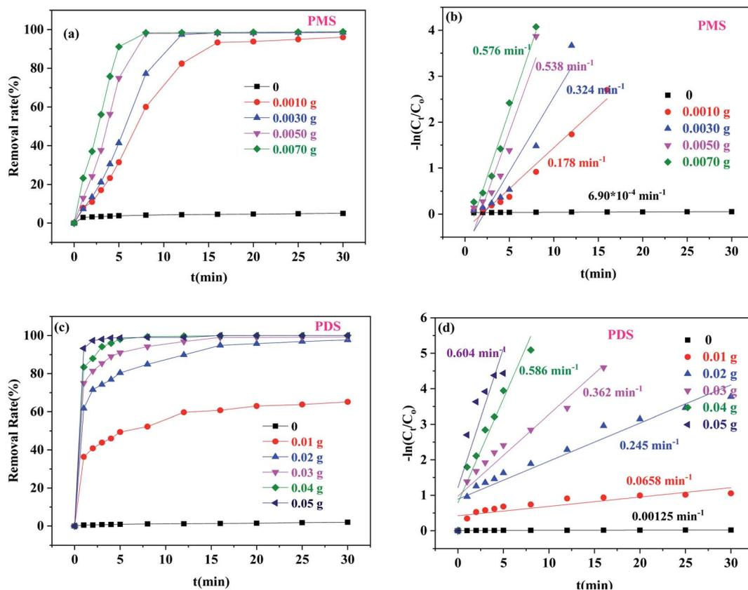
Fig. 5 The effects of Co/C-50 dosage on BPA degradation: removal efficiency of BPA with PMS (a) and PDS (c), and corresponding pseudo-first-order kinetic rate constants (b and d) ([PMS] = 0.25 g L<sup>-1</sup>, [PDS] = 1.0 g L<sup>-1</sup>, [BPA] = 20 mg L<sup>-1</sup>,  $T = 30^\circ\text{C}$ ).
