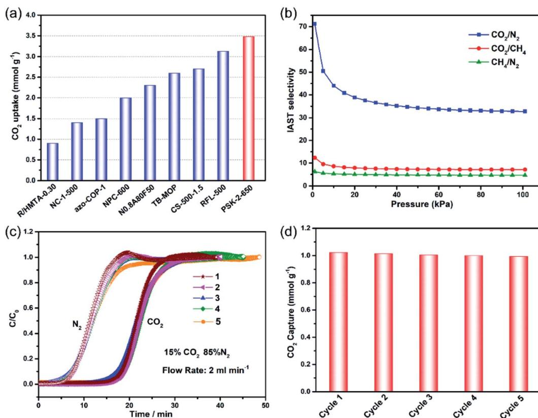
Fig. 4 (a) Comparison of CO<sub>2</sub> uptake among representative porous materials; (b) IAST selectivity of CO<sub>2</sub>/N<sub>2</sub> (15 : 85), CO<sub>2</sub>/CH<sub>4</sub> (10 : 90) and CH<sub>4</sub>/N<sub>2</sub> (50 : 50) on PSK-1-550 at 298 K; (c) the breakthrough experiments of PSK-2-650 for CO<sub>2</sub>/N<sub>2</sub> mixture (15/85, v/v) with a gas flow of 2 mL min<sup>-1</sup>, (d) cyclic CO<sub>2</sub> adsorption capacity.
