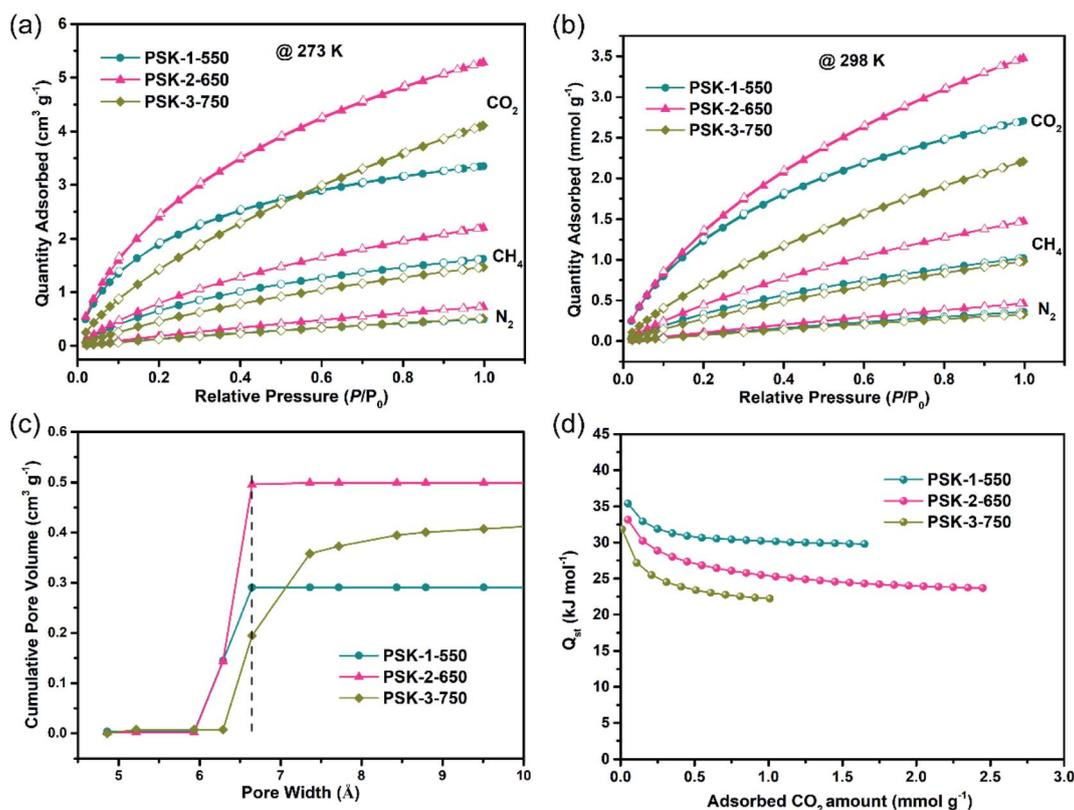
Fig. 3 CO<sub>2</sub>, CH<sub>4</sub>, N<sub>2</sub> adsorption isotherms (a) at 273 K and (b) at 298 K, (c) cumulative pore volume derived from N<sub>2</sub> adsorption at 77 K, (d) isosteric heat of CO<sub>2</sub> adsorption.
