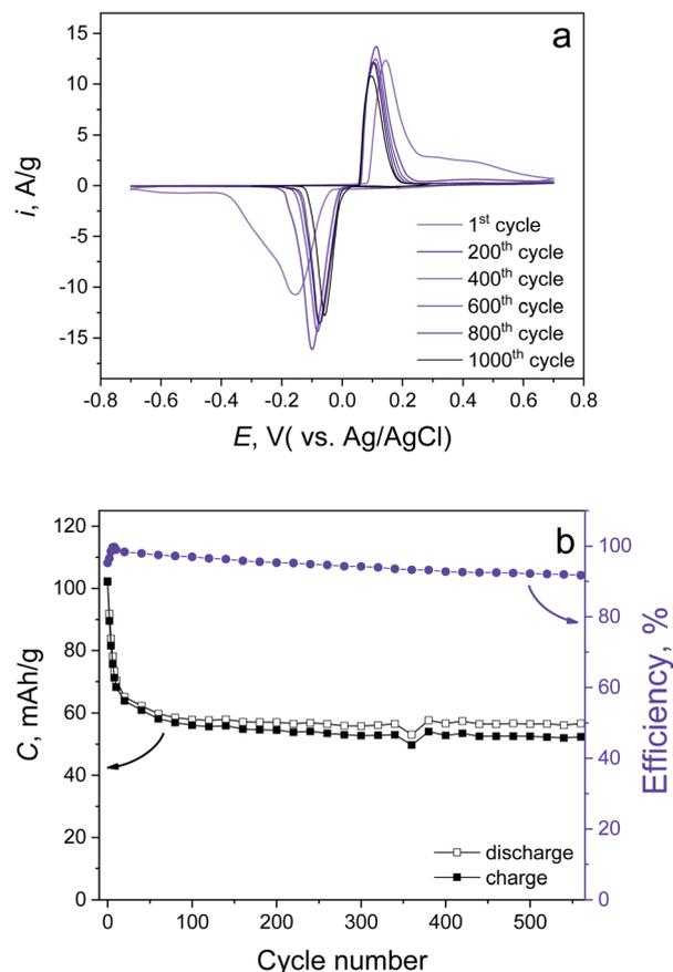
Fig. 4 Cycling stability tests of the synthesized material performed by (a) CV mode at 5 mV s<sup>-1</sup> and (b) GC mode at 1 A g<sup>-1</sup>.
