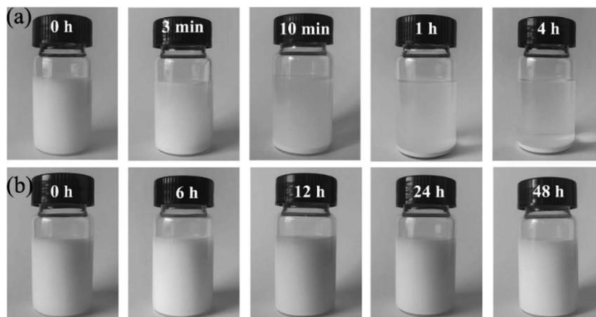
Fig. 3 Photographs of sedimentation process of (a) unmodified ZrO<sub>2</sub> and (b) APTES-modified ZrO<sub>2</sub> dispersed in anhydrous alcohol at different times.
