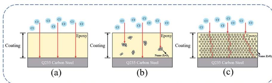
Fig. 9 Corrosion protection mechanism of coatings: (a) pure epoxy, (b) 3–4 wt% zirconia, (c) 1–2 wt% zirconia.
