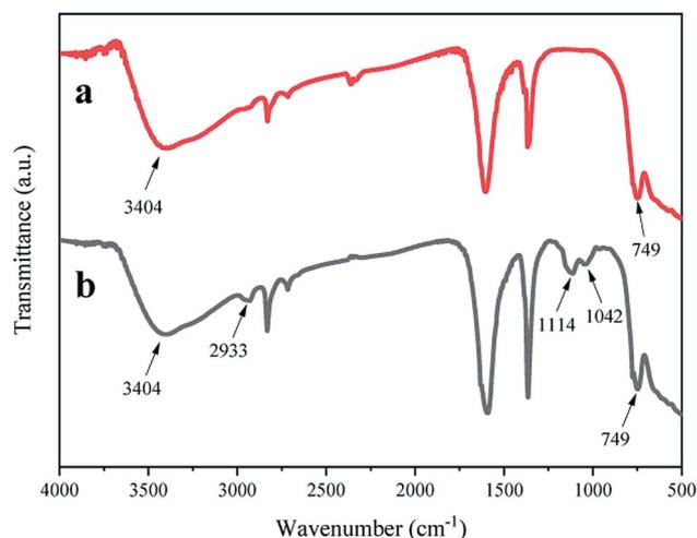
Fig. 2 FTIR spectra of untreated (a) and APTES-modified (b) ZrO<sub>2</sub> nanoparticles.
