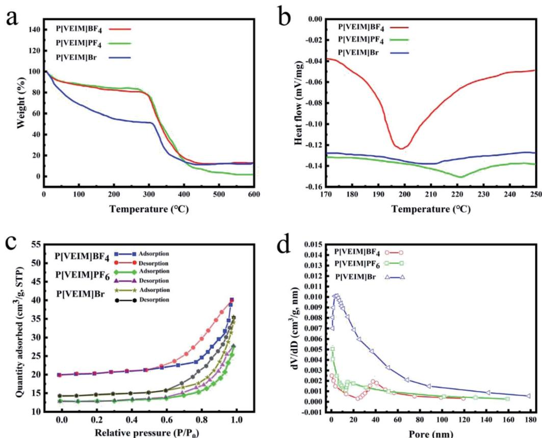
Fig. 5 Characterization of PILs. (a) TGA; (b) DSC; (c) N<sub>2</sub> adsorption–desorption curves; (d) distribution of pore size.
