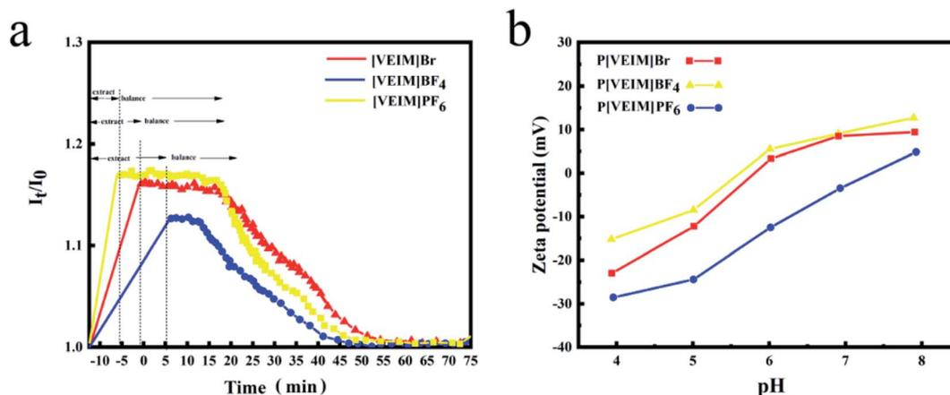
Fig. 9 (a) The formation and reintegration of hydrogen bonds; (b) zeta potential of PILs at varying solution pH. *I*<sub>0</sub> indicates the O–H vibration intensity before extraction; and *I*<sub>*t*</sub> denotes the O–H vibration intensity at *t* time after extraction by PILs.
