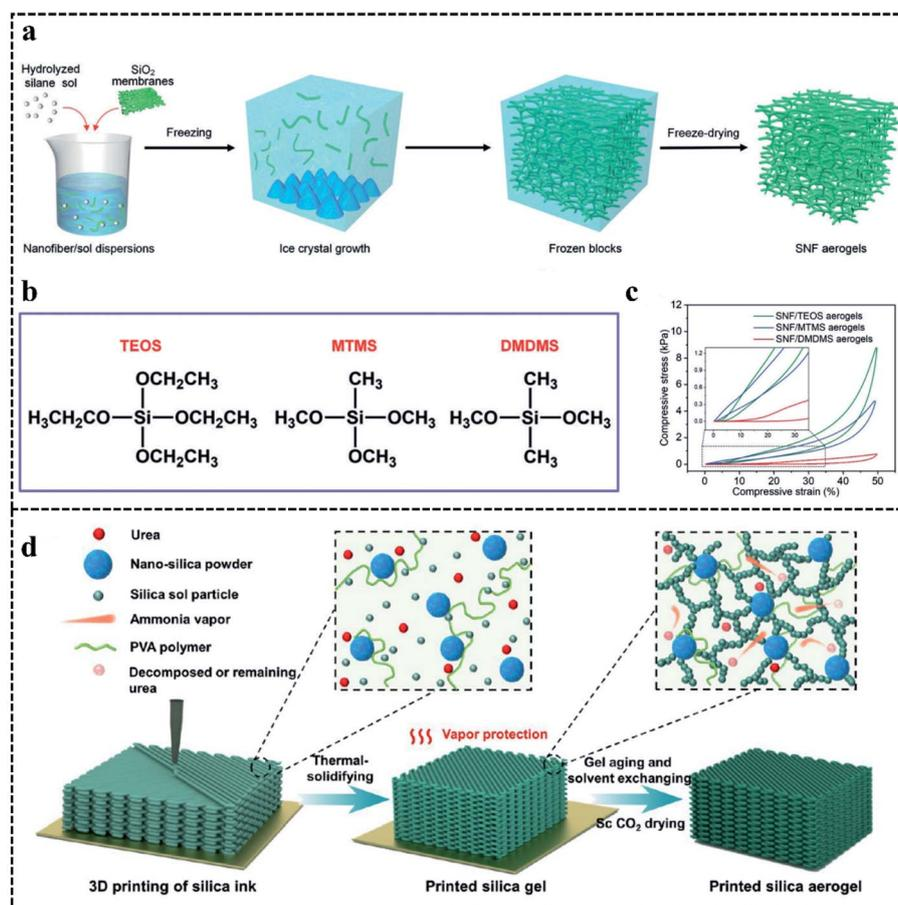
Fig. 4 (a) Synthetic route of SNF aerogels. (b) Structures of different crosslinking silane coupling agents. (c) Compressive  $\sigma$  versus  $\epsilon$  at the 5th loading–unloading cycle of different SNF aerogels.<sup>121</sup> Copyright 2020, John Wiley and Sons. (d) Synthetic route of thermal-solidifying SAs.<sup>58</sup> Copyright 2021, American Chemical Society.
