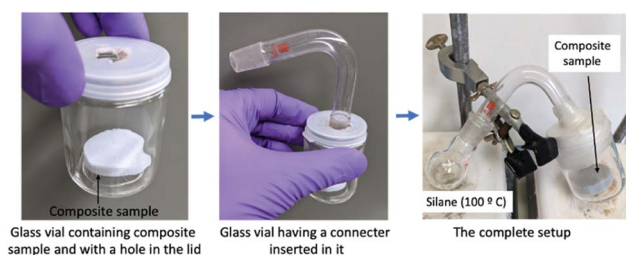
Fig. 1 Steps used to make a vapor phase hydrophobic coating on the composite sample.
