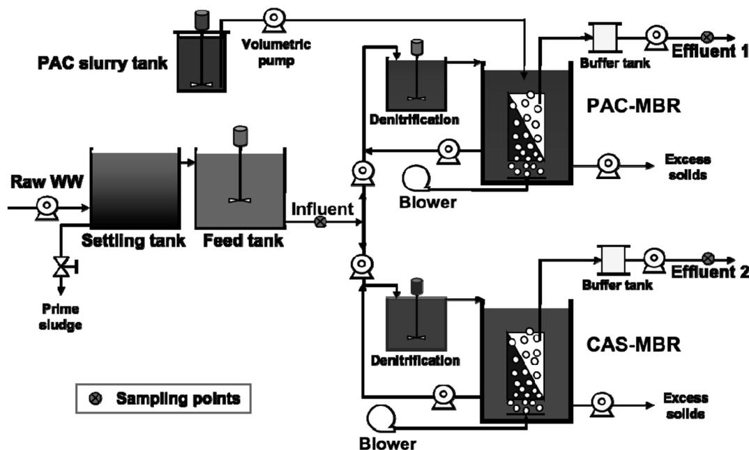
Fig. 1 Schematic diagram of the experimental setup.
