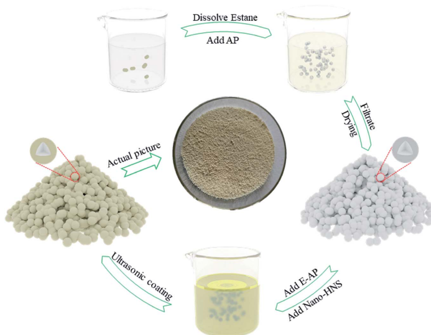
Fig. 1 The preparation process of core-shell AP@HNS composites.
