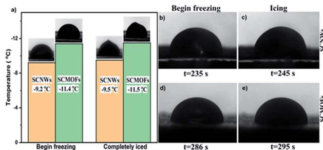
Fig. 3 (a) Freezing point of SCNWs and SCMOFs. Freezing process of water droplets at  $-20^\circ\text{C}$ , (b and c) the droplet is on the surface of SCNWs; (d and e) the droplet is on the surface of SCMOFs.
