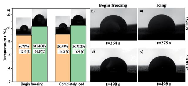
Fig. 5 (a) Freezing point of SCNWs and SCMOFs under the light irradiation. Freezing process of water droplets at  $-20\text{ }^{\circ}\text{C}$  under the light irradiation, (b and c) the droplet is on the surface of SCNWs; (d and e) the droplet is on the surface of SCMOFs.
