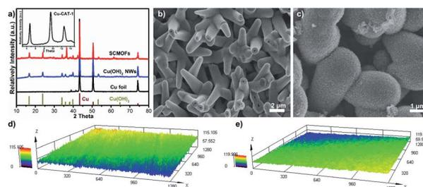
Fig. 1 (a) X-ray diffraction patterns of Cu foil,  $Cu(OH)_2$  NWs and SCMOFs. Scanning electron microscopy images of  $Cu(OH)_2$  NWs (b) and Cu-CAT-1 (c). The confocal laser scanning microscopy images of Cu-CAT-1 (d) and SCMOFs (e).
