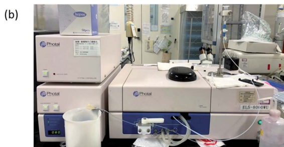
Fig. 2 Zeta potential and measurement method. (a) Zeta potential model; (b) zeta potential measurement unit used in the experiment.
