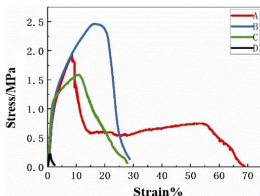
Fig. 4 Shows the stress-strain curves of sandwich structure, insulation layer, slow release layer, and quick release layer A, B, C, and D in sequence.
