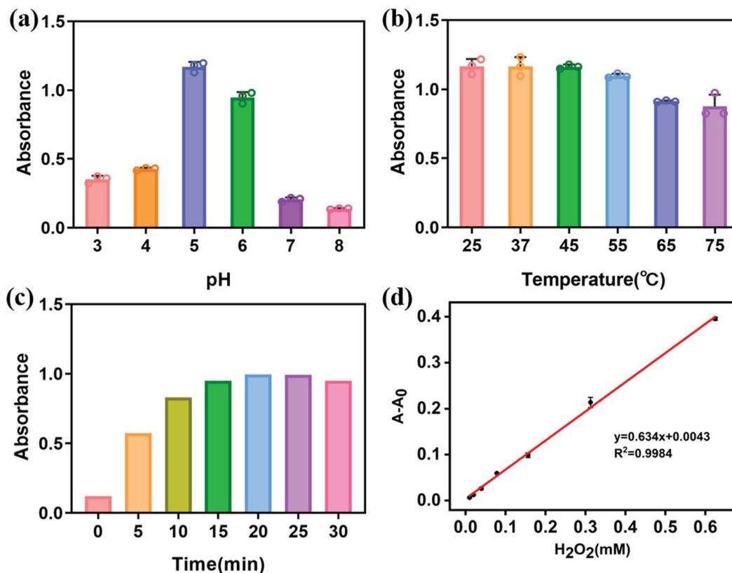
Fig. 5 Optimization of variable experimental factors of colorimetric detection; (a) pH; (b) reaction temperature; (c) reaction time; (d) the linear range of H<sub>2</sub>O<sub>2</sub> colorimetric detection. Error bars represent the standard deviation of three repeated measurements.
