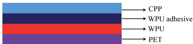
Fig. 2 Schematic diagram of PET/CPP laminate film samples for the measurements of T-peel.
