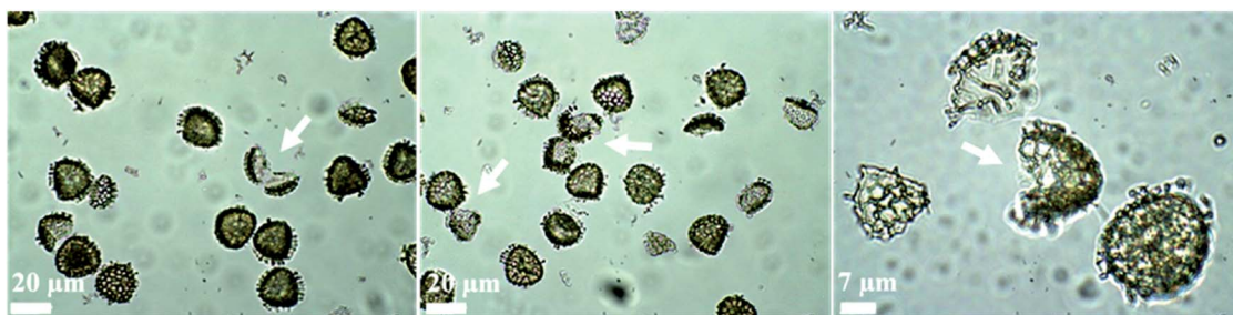
Fig. 3 Optical pictures of ultrasonically shattered ASA-loaded LCS microcapsules at various magnifications following the last sonication cycle used to extract ASA for loading capacity tests. The ASA-loaded LCS were subjected to a four-cycle sonication technique, and each cycle consists of two minutes of sonication at 50% amplitude three times. Some sporopollenin ornaments are fragmented (indicated by arrows).
