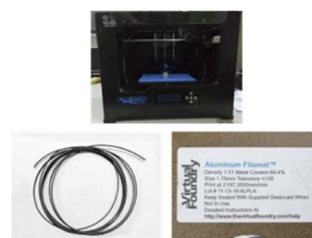
Fig. 2 3D printer and filament used to fabricate the scaffold.
