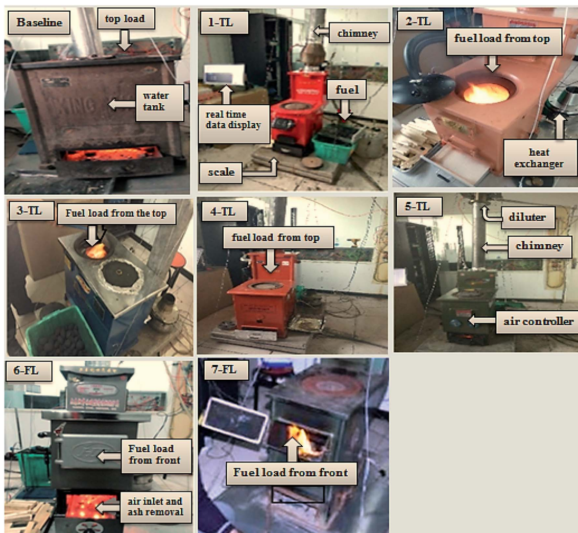
Fig. 2 Stoves used in the current study with different feeding method and design.
