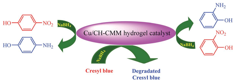
Scheme 7 Degradation of 2-NP, 4-NP and CB by Cu/CS-CMM catalyst.
