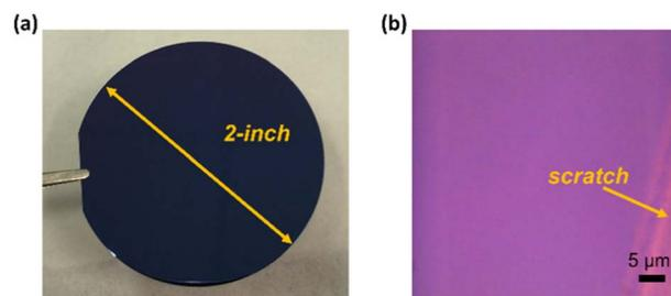
Fig. 2 Monolayer WS<sub>2</sub> films grown on SiO<sub>2</sub>/Si substrates. (a) Photo of a 2 inch wafer covered with a WS<sub>2</sub> monolayer; (b) microscope image of the WS<sub>2</sub> monolayer with an intentional scratch.
