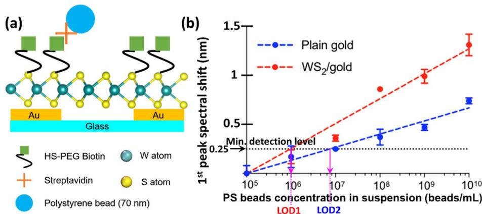
**Fig. 7** (a) Schematic representation of our WS<sub>2</sub>-Au nanohole array SPR immunosensor functionalized with biotin and tested using streptavidin-coated PS beads. (b) Measured optical spectral shift for the central wavelength of the first transmission peak as a function of the streptavidin-coated PS beads concentration for plain and WS<sub>2</sub>-coated Au nanohole arrays sensors functionalized with biotin.
