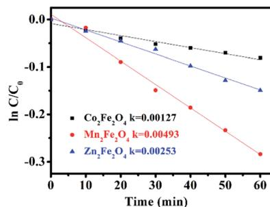
Fig. 6 First-order plots for the photocatalytic degradation of LVX using MFe<sub>2</sub>O<sub>4</sub>.
