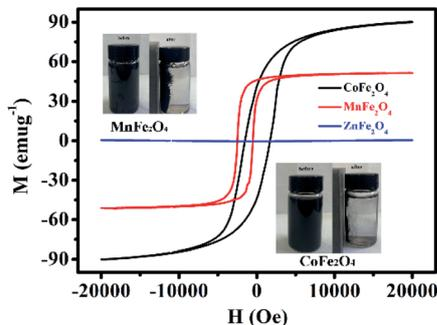
Fig. 5 Magnetic hysteresis loops of MFe<sub>2</sub>O<sub>4</sub>. The inset shows photos of well-dispersed MFe<sub>2</sub>O<sub>4</sub> in water and magnetic separation of MFe<sub>2</sub>O<sub>4</sub>.
