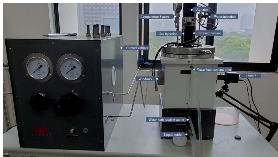
Fig. 2 Schematic of the high-pressure hydrate reactor system.
