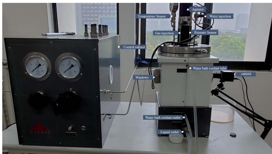
Fig. 2 Schematic of the high-pressure hydrate reactor system.
