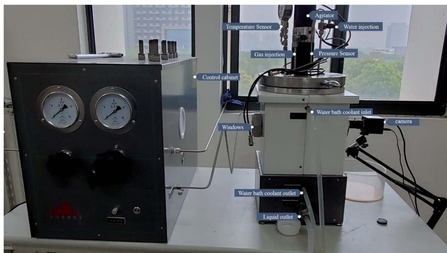
Fig. 2 Schematic of the high-pressure hydrate reactor system.
