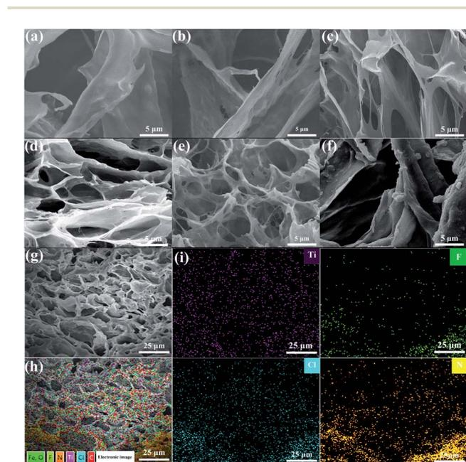
Fig. 1 SEM images of PVA/QCS-C/MXene hydrogels with different QCS-C contents. (a) PVA/QCS-C<sub>5</sub>/MXene, (b) PVA/QCS-C<sub>10</sub>/MXene, (c) PVA/QCS-C<sub>15</sub>/MXene, (d) PVA/QCS-C<sub>20</sub>/MXene, (e) PVA/QCS-C<sub>25</sub>/MXene, (f) PVA/QCS-C<sub>30</sub>/MXene, (g) SEM image of PVA/QCS-C<sub>15</sub>/MXene after  $\text{FeCl}_3$  cross-linking, (h) and (i) EDS images of (g).
