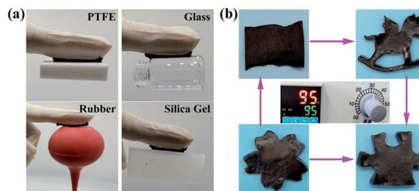
Fig. 4 (a) Digital photos of the hydrogel adhered to the surface of different substrates. (b) Re-modelling the hydrogel into different morphologies after dissolved into aqueous solution at  $95 \text{ }^\circ\text{C}$ .
