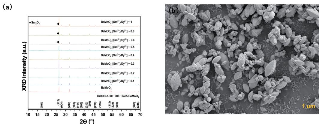
Fig. 4 (a) XRD patterns of  $\text{BaMoO}_4\text{:}[\text{Sm}^{3+}]/[\text{Dy}^{3+}]$  according to  $\text{Sm}^{3+}$  ion concentration and (b) FE-SEM image of  $\text{BaMoO}_4\text{:}[\text{Sm}^{3+}]/[\text{Dy}^{3+}]$ .
