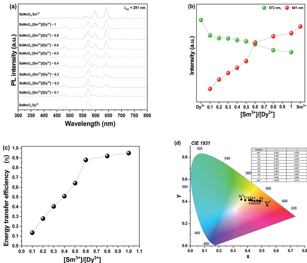
Fig. 5 BaMoO<sub>4</sub>:[Sm<sup>3+</sup>]/[Dy<sup>3+</sup>] of (a) PL spectra under 291 nm, (b) change of 572 nm (Dy<sup>3+</sup>) and 641 nm (Sm<sup>3+</sup>), (c) energy transfer efficiency, and (d) CIE coordinate of the BaMoO<sub>4</sub> phosphors.
