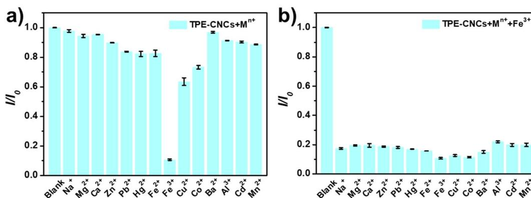
Fig. 1 (a) Fluorescence response of TPE-CNCs aqueous suspensions (0.05 wt%) to various metal ions (300  $\mu\text{M}$ ). (b) Fluorescence response of TPE-CNCs aqueous suspensions (0.05 wt%) to  $\text{Fe}^{3+}$  in the presence of competition metal ions (300  $\mu\text{M}$ ) ( $\lambda_{\text{ex}} = 330 \text{ nm}$ , Ex/Em = 6/4) ( $I_0$  and  $I$  are the fluorescence intensities of TPE-CNCs without and with metal ions).
