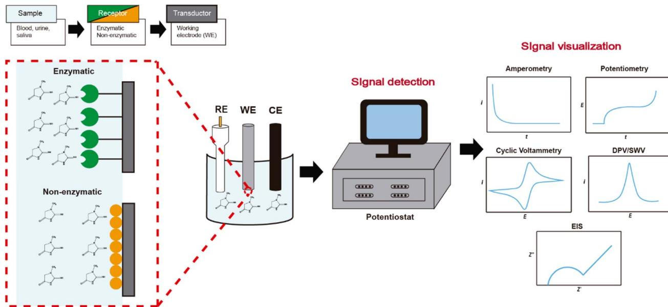
Fig. 3 Schematic representation of electrochemical creatinine detection and signal visualization with different electrochemical techniques (amperometry, potentiometry, cyclic voltammetry, differential pulse voltammetry, square wave voltammetry, electrochemical impedance spectroscopy).
