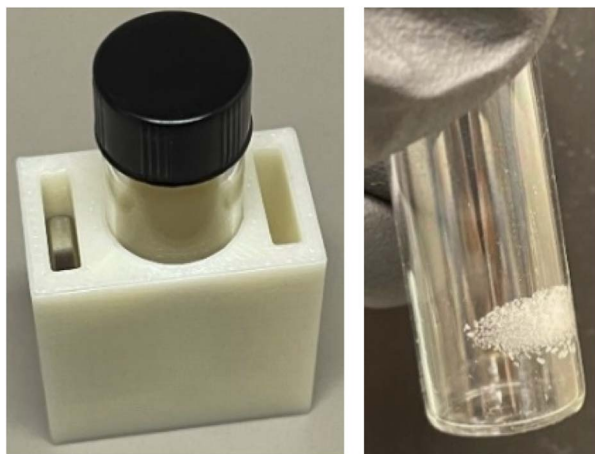
Fig. 2 Left: 3D printed holder containing the binary mixture of RE elements at 2 mm distance to a \text{Fe}_{14}\text{Nd}_2\text{B} magnet. Right: Crystals formed near the magnet after holding the binary mixture solution at the magnet for 72 h at 3 °C.
