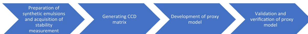
Fig. 1 Steps for developing a proxy model for the prediction of emulsion stability.
