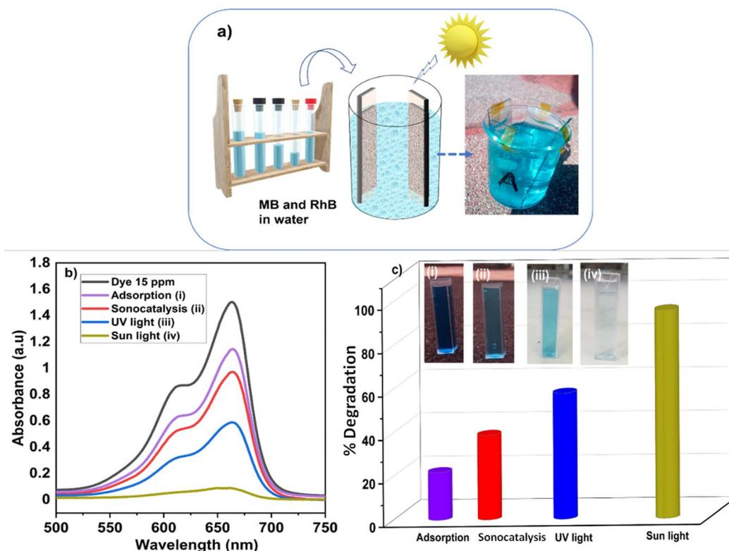
Fig. 4 (a) Methylene blue degradation mechanism under solar light-driven NiO NWs as a photocatalyst, (b) UV-Vis absorbance spectra of several techniques for removing methylene blue dye from aquatic environments, and (c) its bar chart depiction with insets of real-time images containing MB dye degradation.
