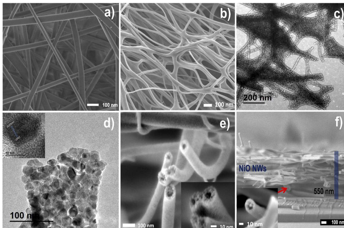
Fig. 3 (a) FESEM analysis of (a) PVA/ $\text{Ni}(\text{NO}_3)_2$  nanofiber composite, (b) NiO NWs after calcination at 450 °C, (c and d) TEM pictures of NiO NWs at various magnifications inset of the HRTEM (10 nm) pattern, (e) hollow morphology of NiO NWs with the inset of higher magnification, (f) cross-sectional view of hollow NiO NWs, inset showed a higher magnification hollow cross-sectional view.
