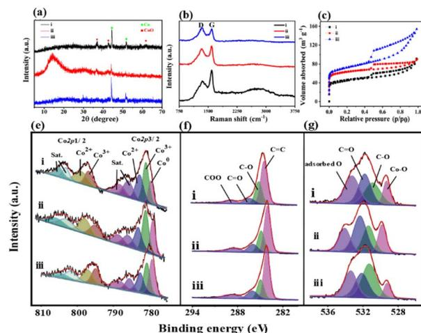
**Fig. 2** (a) XRD patterns, (b) Raman spectra, (c)  $\text{N}_2$  adsorption-desorption isotherms, and the high-resolution (e) Co 2p, (f) C 1s and (g) O 1s XPS spectra of (i)  $\text{Co}/\text{Co}_x\text{O}_y@m\text{C}_{400}$ , (ii)  $\text{Co}/\text{Co}_x\text{O}_y@m\text{C}_{600}$ , and (iii)  $\text{Co}/\text{Co}_x\text{O}_y@m\text{C}_{800}$ .
