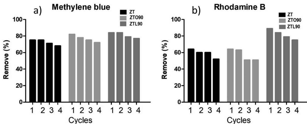
Fig. 9 (a) Effect of desorption cycles on methylene blue removal (MB concentration = 200 mg L<sup>-1</sup>, nanoparticles content = 20 mg/100 mL,  $T = 25^\circ\text{C}$  and 12 min) or (b) rhodamine B (concentration = 200 mg L<sup>-1</sup>, nanoparticles 20 mg/100 mL and  $t = 12$  min).
