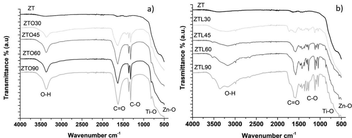
Fig. 1 FTIR spectra of (a) ZTO and (b) ZTL.
