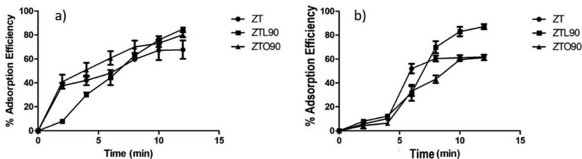
Fig. 8 (a) The adsorption efficiency of ZT, ZTL90 and ZTO90 (MB concentration = 200 mg L<sup>-1</sup>, nanoparticles content = 20 mg/20 mL,  $T = 25^\circ\text{C}$  and 12 min). (b) The adsorption efficiency of ZT, ZTL90 and ZTO90 (rhodamine B concentration = 200 mg L<sup>-1</sup>, nanocomposite content = 20 mg/20 mL,  $T = 25^\circ\text{C}$  and 12 min).
