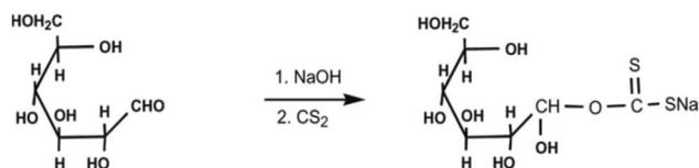
Scheme 2 Inferred mechanism for the xanthation of CSB to give CXSB.<sup>2</sup>
