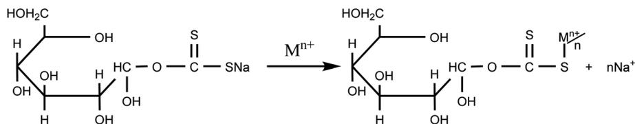
Scheme 3 Plausible adsorption mechanism of  $M^{n+}$ (Hg) ion onto monomeric cellulose unit contained in CXSB.<sup>2</sup>
