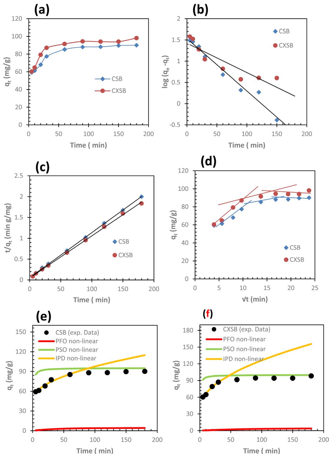
Fig. 6 Biosorption kinetics of Hg(II) onto CSB and CXSB (a) experimental plot, (b–d) linear fitting of kinetic data using PFO, PSO and IPD models, and (e and f) non-linear fitting of kinetic data using PFO, PSO and IPD models.
