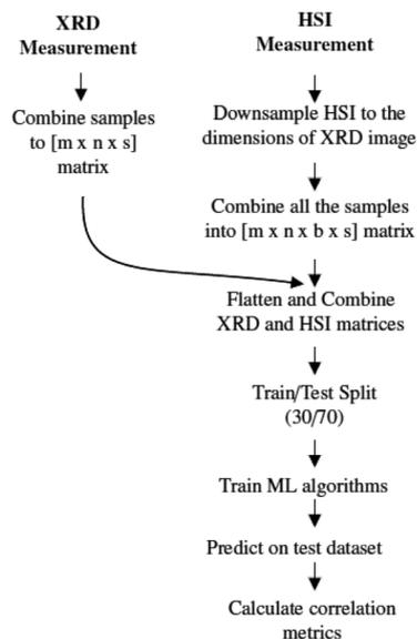
Fig. 6 Flow chart of the steps to compare XRD and HSI measurement. This is done for each investigated mineral. With  $m$  and  $n$  as the horizontal and pixels dimensions,  $s$  as the number of samples and  $b$  the number of spectral bands.
