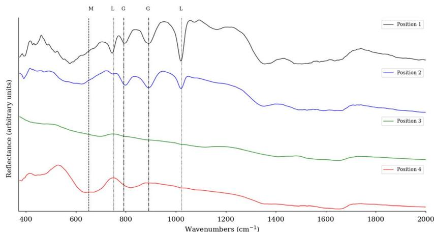
Fig. 7 FTIR Reflectance spectra for four different positions in sample six. The vertical lines represent the distinct features that are described in the literature for each mineral. (G = goethite, M = maghemite, L = lepidocrocite).
