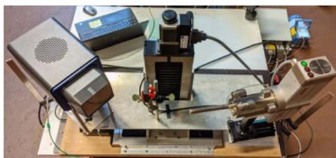
Fig. 4 Image of the scanning XRD setup.
