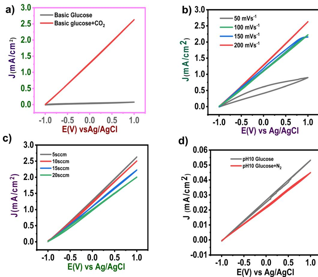
Fig. 3 Cyclic voltammetry plots for glucose cell (a) with and without CO<sub>2</sub> (b) effect of scan rate in CO<sub>2</sub> saturated glucose cell (c) CV curves obtained at different gas flow rates of CO<sub>2</sub> (scan rate 50 mV s<sup>-1</sup>) (d) with and without N<sub>2</sub>.
