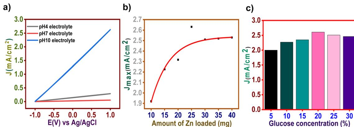
Fig. 4 Evaluation of the performance of CO<sub>2</sub> saturated glucose cell (a) pH effect (b) effect of zinc loading (c) effect of glucose concentration.
