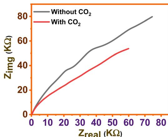
Fig. 6 EIS spectra of CO<sub>2</sub> saturated and unsaturated solution.
