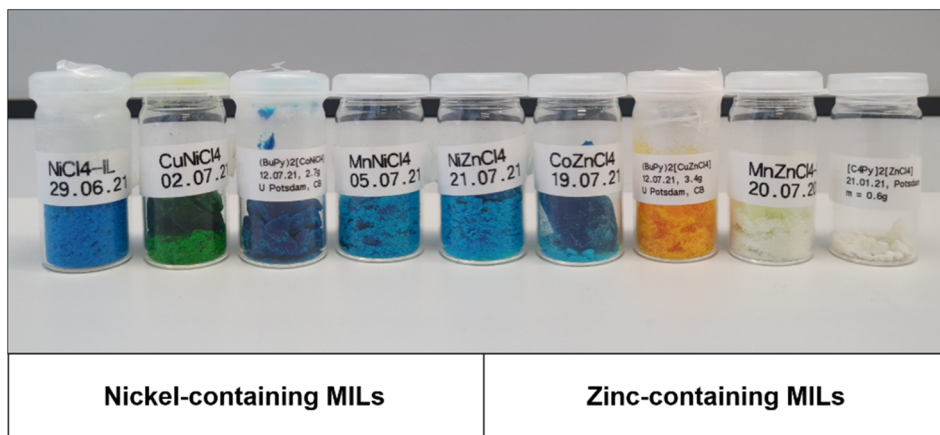
Fig. 1 Ni- and Zn-based mixed metal ILs. Nominal composition is always (C_4Py)_2[Ni_{0.5}M_{0.5}Cl_4] or (C_4Py)_2[Zn_{0.5}M_{0.5}Cl_4] . For precise metal contents see Table 1 below.
