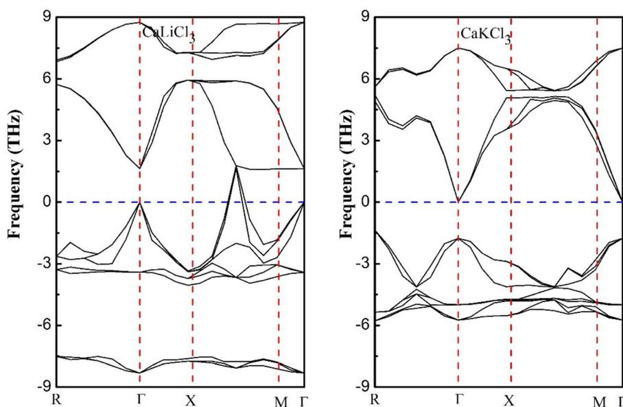
**Fig. 3** Phonon dispersion curves at high symmetries points for ternary CaQCl<sub>3</sub> (Q = Li and K) chloroperovskites compounds.
