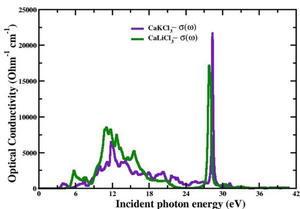
Fig. 6 The computed optical conductivity for CaQCl<sub>3</sub> (Q = Li and K) chloroperovskites.
