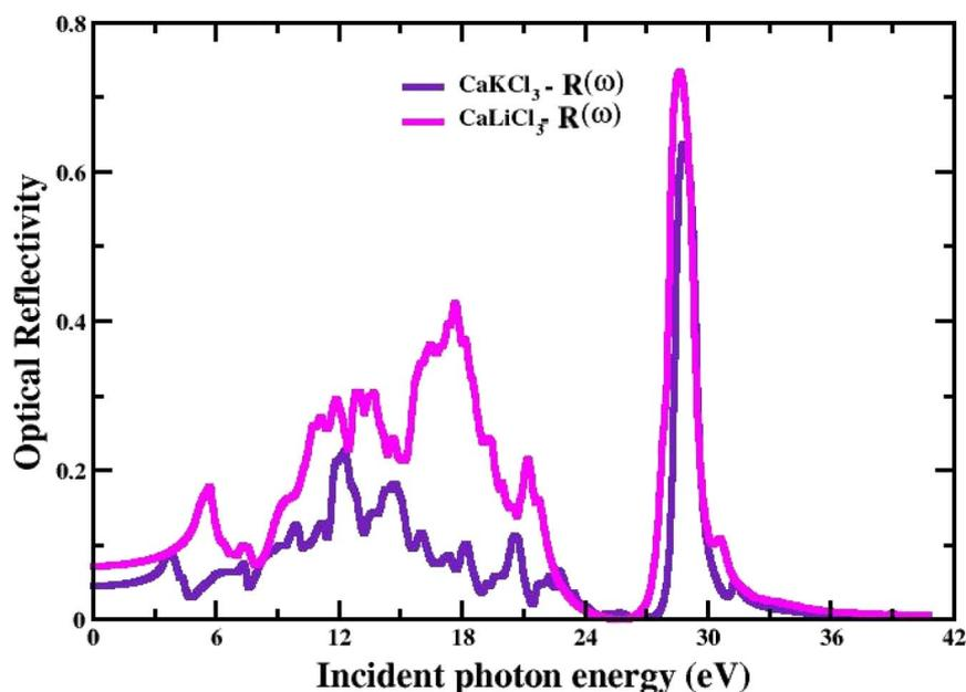
Fig. 10 The computed optical reflectivity for  $\text{CaQCl}_3$  (Q = Li and K) chloroperovskites.
