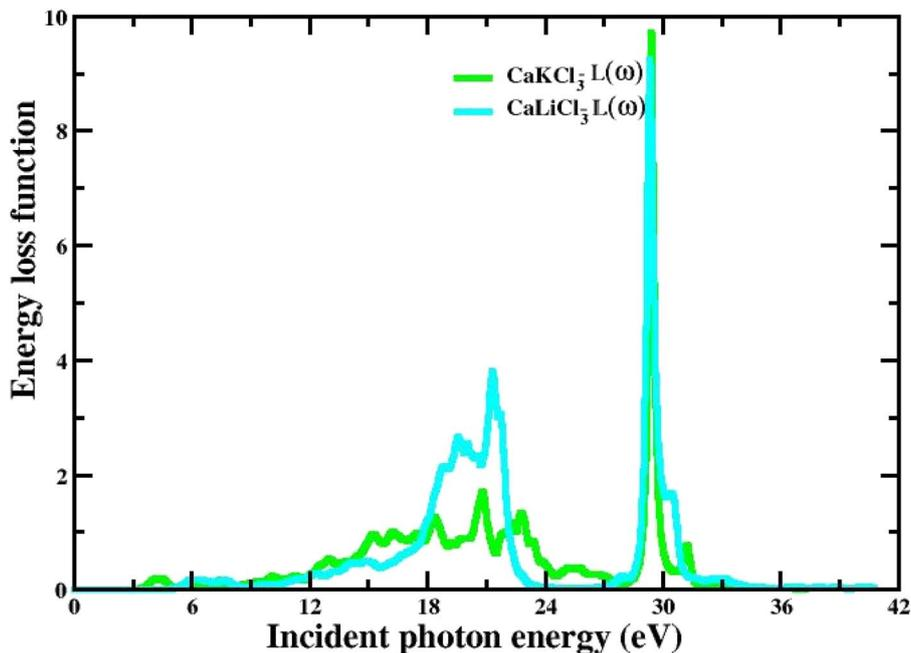
Fig. 11 The computed energy loss function for CaQCl<sub>3</sub> (Q = Li and K) chloroperovskites.
