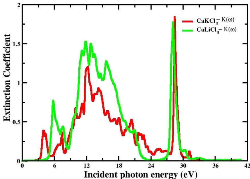
Fig. 8 The computed extinction co-efficient for CaQCl<sub>3</sub> (Q = Li and K) chloroperovskites.
