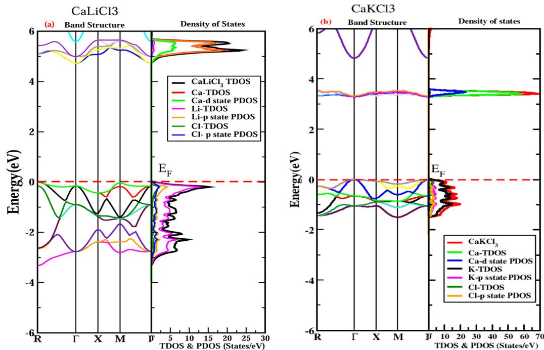
Fig. 4 The examined fitted electronic band structures and DOS for  $\text{CaQCl}_3$  ( $Q = \text{Li}$  and  $\text{K}$ ) chloroperovskites at high symmetries points in the first Brillouin zone using TB-mBJ approximation.
