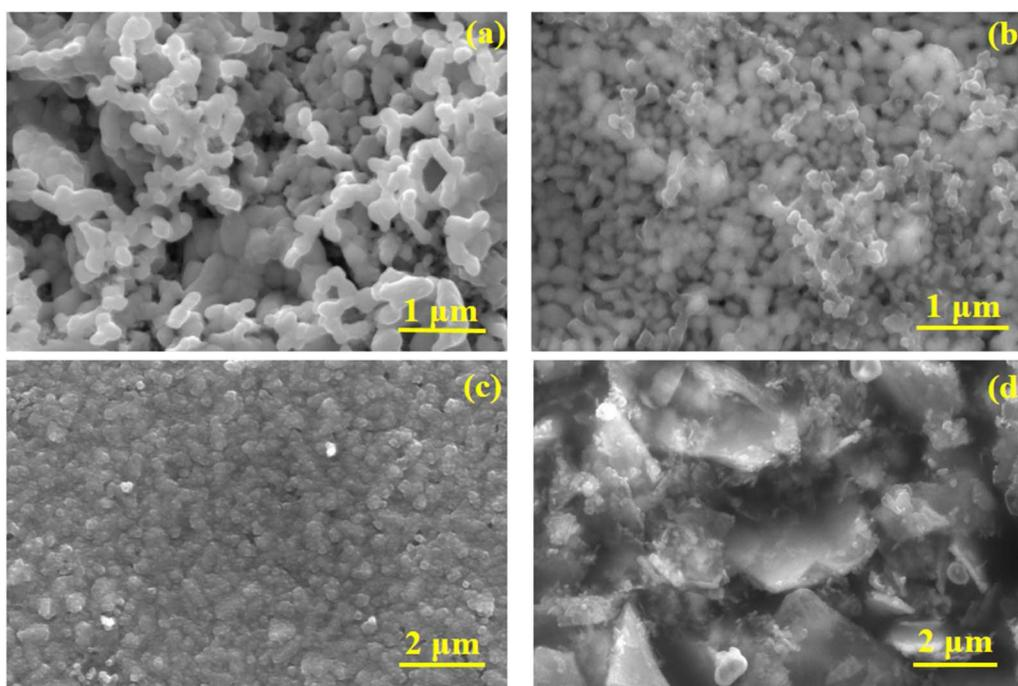
Fig. 3 FESEM micrographs of (a)  $\text{BiVO}_4$  photoanode, (b)  $\text{Mo-BiVO}_4/\text{TiO}_2/\text{FeOOH}$  photoanode, (c)  $\text{Cu}_2\text{O}$  photocathode, (d)  $\text{Cu}_2\text{O}/\text{TiO}_2/\text{MoS}_2$  photocathode.
