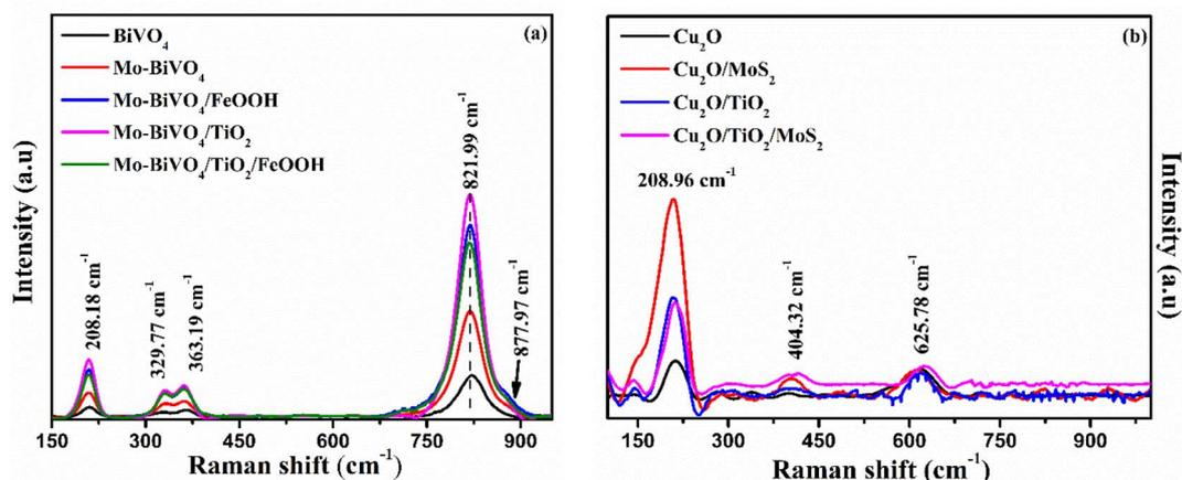
Fig. 2 (a) Raman spectra of  $\text{BiVO}_4$ ,  $\text{Mo-BiVO}_4$ ,  $\text{Mo-BiVO}_4/\text{FeOOH}$ ,  $\text{Mo-BiVO}_4/\text{TiO}_2$  and  $\text{Mo-BiVO}_4/\text{TiO}_2/\text{FeOOH}$  photoanodes and (b) Raman spectra of  $\text{Cu}_2\text{O}$ ,  $\text{Cu}_2\text{O}/\text{MoS}_2$ ,  $\text{Cu}_2\text{O}/\text{TiO}_2$  and  $\text{Cu}_2\text{O}/\text{TiO}_2/\text{MoS}_2$  photocathodes.
