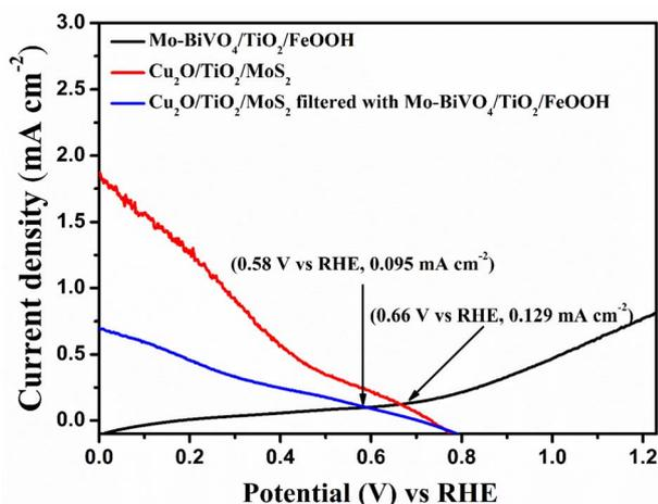
Fig. 7 Overlaid LSV Plot of Mo-BiVO<sub>4</sub>/TiO<sub>2</sub>/FeOOH photoanode with Cu<sub>2</sub>O/TiO<sub>2</sub>/MoS<sub>2</sub> photocathode and Cu<sub>2</sub>O/TiO<sub>2</sub>/MoS<sub>2</sub> photocathode filtered by Mo-BiVO<sub>4</sub>/TiO<sub>2</sub>/FeOOH photoanode.
