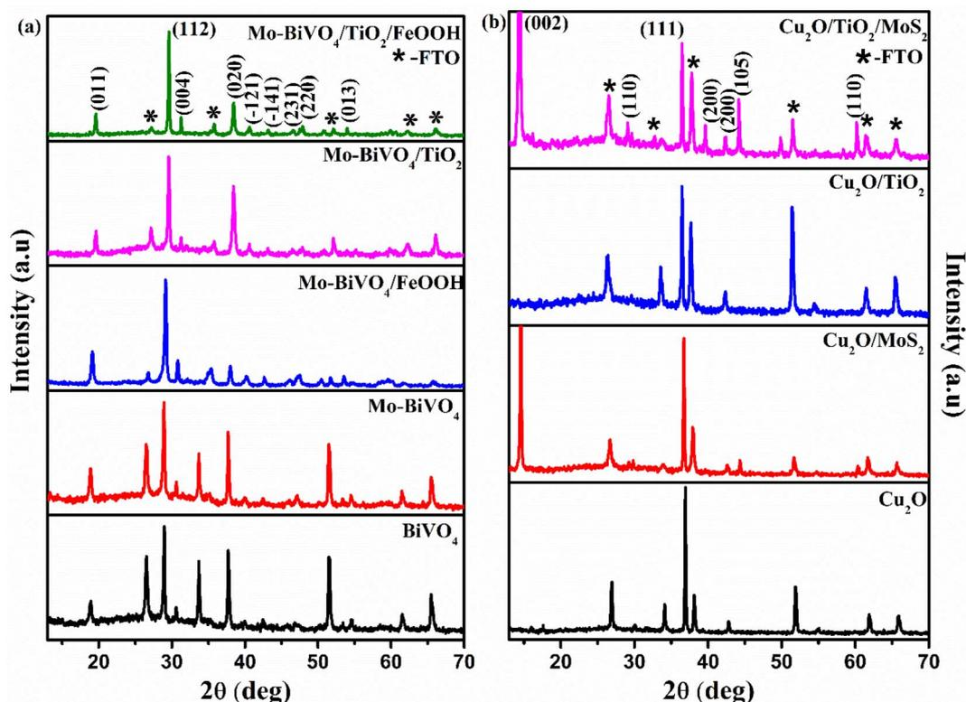
Fig. 1 (a) X-ray diffraction spectra of  $\text{BiVO}_4$ ,  $\text{Mo-BiVO}_4$ ,  $\text{Mo-BiVO}_4/\text{FeOOH}$ ,  $\text{Mo-BiVO}_4/\text{TiO}_2$  and  $\text{Mo-BiVO}_4/\text{TiO}_2/\text{FeOOH}$  photoanodes (b) X-ray diffraction spectra of  $\text{Cu}_2\text{O}$ ,  $\text{Cu}_2\text{O}/\text{MoS}_2$ ,  $\text{Cu}_2\text{O}/\text{TiO}_2$  and  $\text{Cu}_2\text{O}/\text{TiO}_2/\text{MoS}_2$  photocathodes.
