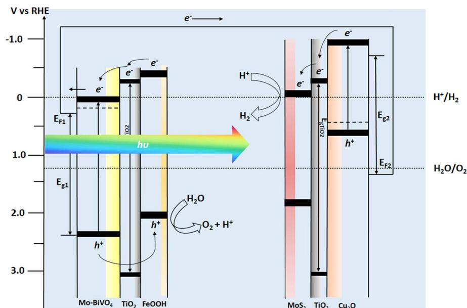
Fig. 8 Energy band diagram of BiVO<sub>4</sub>-Cu<sub>2</sub>O tandem photoelectrochemical cell with respect to RHE potential.
