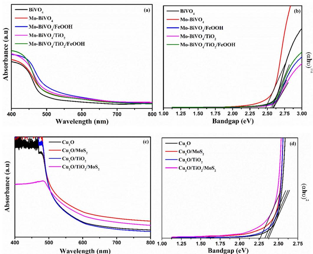
Fig. 4 (a) UV-vis absorption spectra and (b) Tauc plot of BiVO<sub>4</sub>, Mo-BiVO<sub>4</sub>, Mo-BiVO<sub>4</sub>/FeOOH, Mo-BiVO<sub>4</sub>/TiO<sub>2</sub> and Mo-BiVO<sub>4</sub>/TiO<sub>2</sub>/FeOOH photoanodes, (c) UV-vis absorption spectra and (d) Tauc plot of Cu<sub>2</sub>O, Cu<sub>2</sub>O/MoS<sub>2</sub>, Cu<sub>2</sub>O/TiO<sub>2</sub>, Cu<sub>2</sub>O/TiO<sub>2</sub>/MoS<sub>2</sub> photocathodes.
