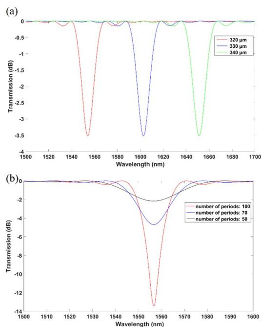
Fig. 2 (a) Simulated transmission spectra of LPFGs with an index modulation of  $1.3 \times 10^{-5}$  and a grating length of 100 periods calculated for three different grating periods:  $\Lambda = 320, 330,$  and  $340 \mu\text{m}$ ; (b) transmission spectra of LPFGs with  $\Lambda = 320 \mu\text{m}$  and an index modulation of  $2.1 \times 10^{-5}$  calculated for three different period lengths: 100, 70, and 50 periods.
