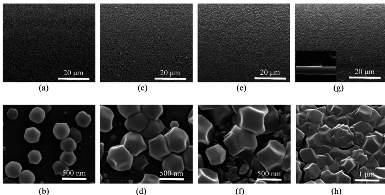
Fig. 4 SEM images of the fiber surface after (a, b) one cycle, (c, d) two cycles, (e, f) three cycles, and (g, h) five cycles (inset: bare fiber with a diameter of  $125 \mu\text{m}$ ) of *in situ* growth of ZIF-8.
