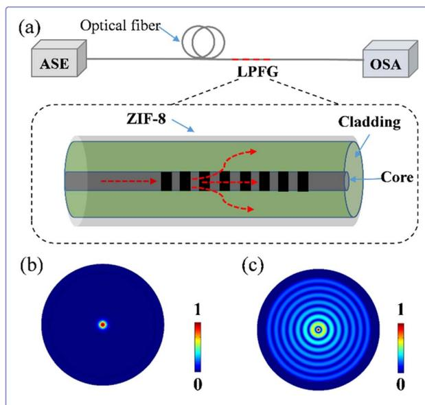
Fig. 1 (a) LPFG coated with ZIF-8 for VOC sensing, where light is launched into the fiber with an ASE source and detected with an OSA; (b) normalized optical intensity distributions of the LP<sub>01</sub> core mode and (c) the LP<sub>08</sub> cladding mode in the fiber.
