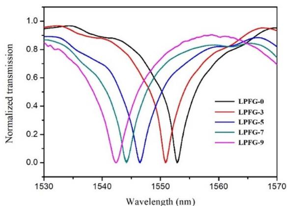
Fig. 5 Transmission spectra of the LPFG before ZIF-8 growth (LPFG-0) and after three (LPFG-3), five (LPFG-5), seven (LPFG-7), and nine (LPFG-9) cycles of ZIF-8 growth.
