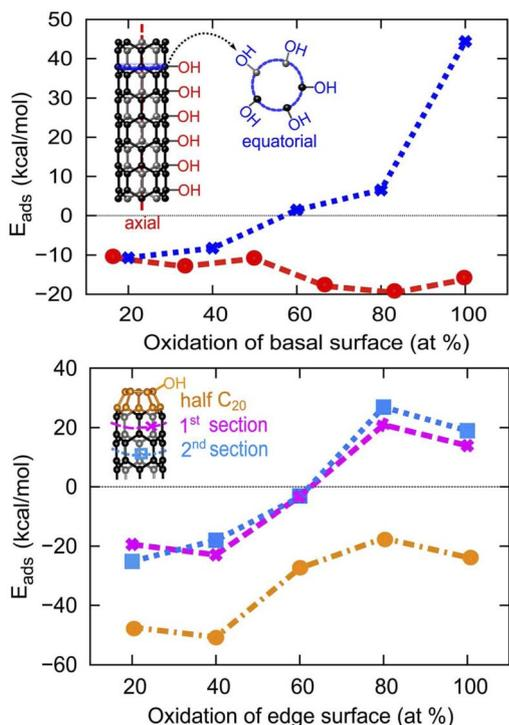
Fig. 5 The evolution of H<sub>2</sub>O adsorption energy at different coverage density on the basal and armchair edge surfaces of SWCNT (5,0), where both edges are capped by half fullerene C<sub>20</sub>.
