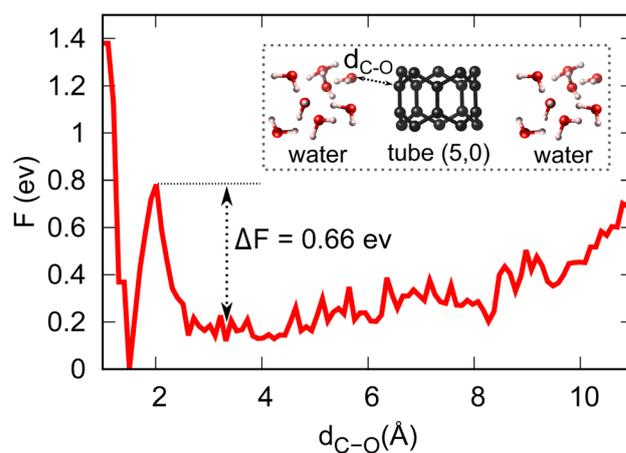
**Fig. 3** Energy profile and activation barrier of H<sub>2</sub>O splitting on the surface of tube (5,0) obtained from metadynamics simulations at  $T = 298.15 \text{ K}$ .
