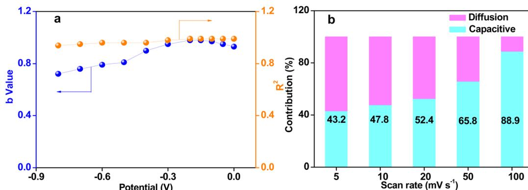
Fig. 7  $b$  values plotted against the potential of the supercapacitor and  $R^2$  values are the corresponding fitting variance (a) and columnar contribution map of surface control capacitance at different scan rates (b).
