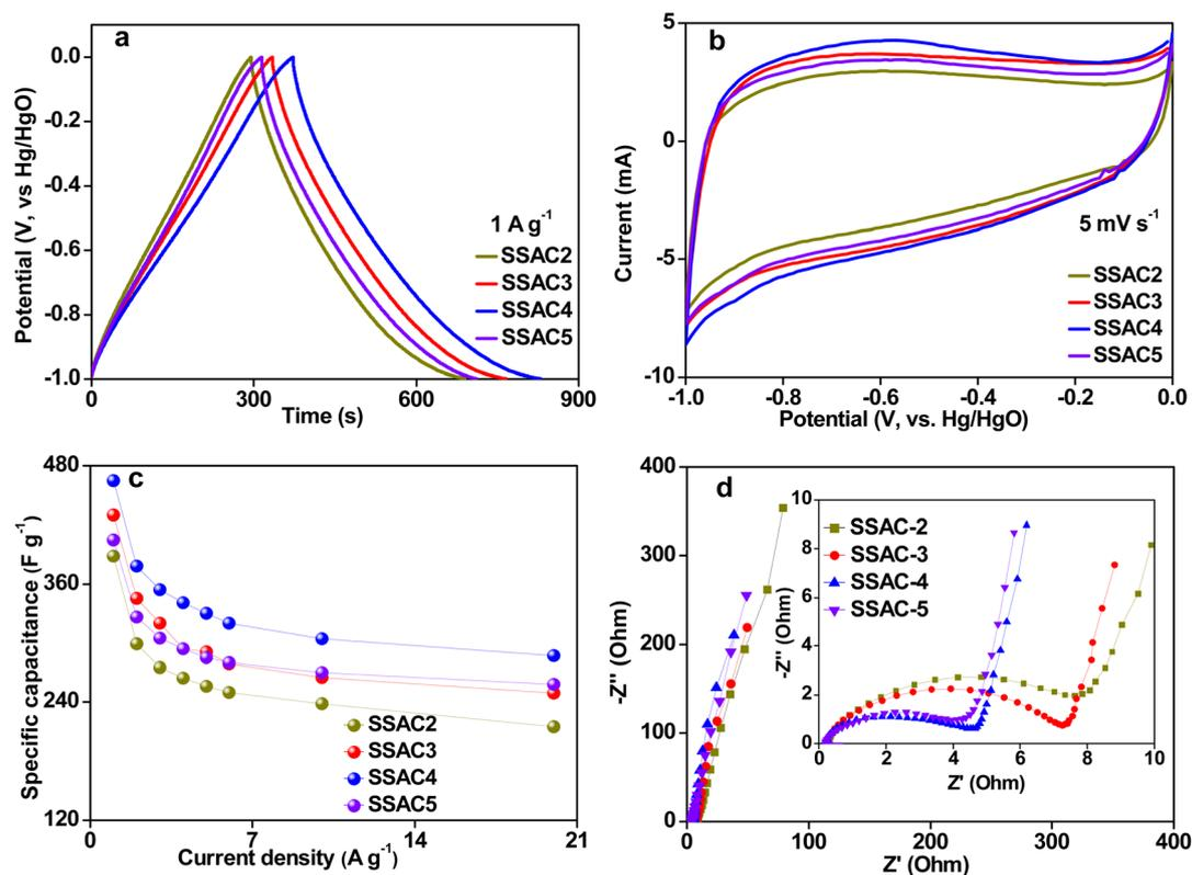
Fig. 6 Electrochemical performance of SSAC $n$  measured using a three-electrode system in 6 M KOH electrolyte. GCD curves at a current density of 1 A g<sup>-1</sup> (a), CV curves at a scan rate of 5 mV s<sup>-1</sup> (b), the  $C_{sp}$  of SSAC $n$  at different current densities (c), and Nyquist plots (d).
