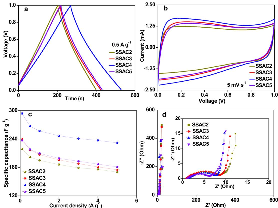
Fig. 8 Electrochemical performance of SSAC $n$  in the all-solid-state supercapacitors in PVA/KOH electrolyte. GCD curves at  $0.5 \text{ A g}^{-1}$  (a), CV curves at  $5 \text{ mV s}^{-1}$  (b), the specific capacitance at different current densities (c), and Nyquist plots (d).
