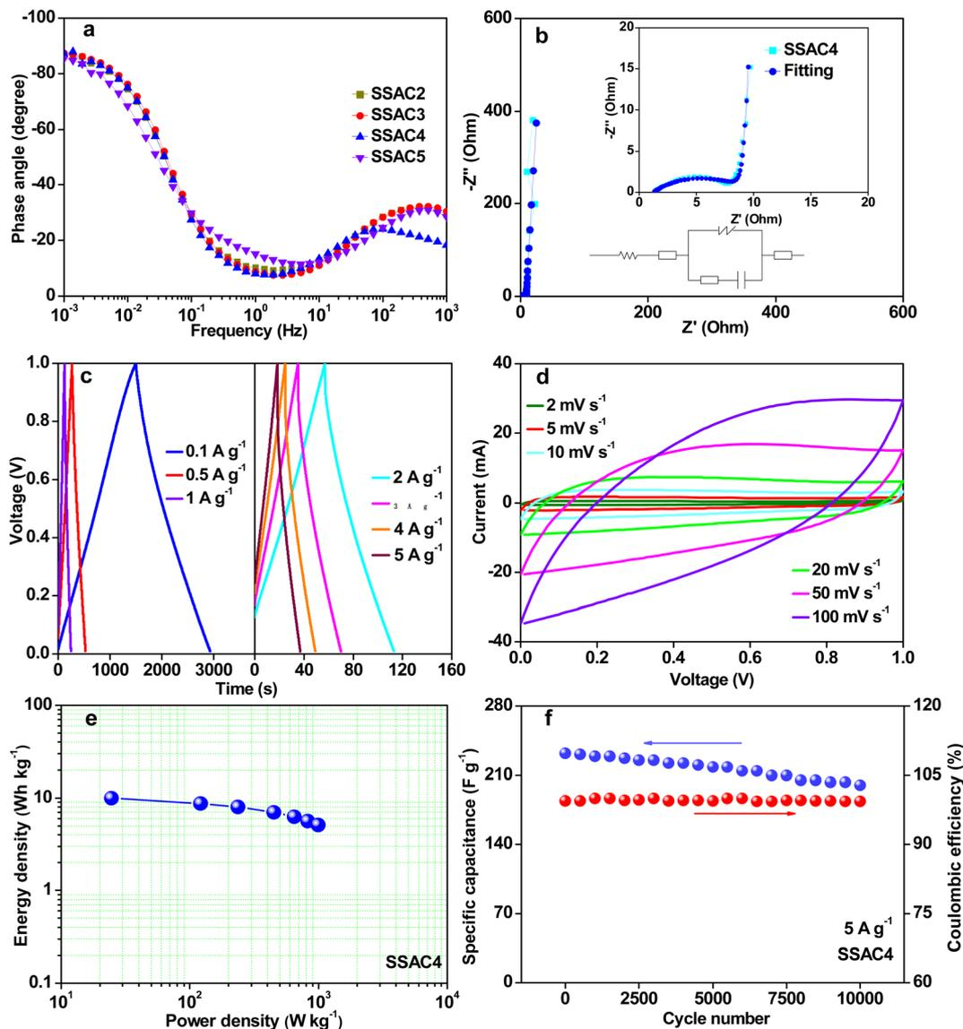
Fig. 9 The Bode plot of SSAC $n$  (a), Nyquist plots (insert is the equivalent circuit model) (b), GCD curves at current densities from 0.1 to 5 A g $^{-1}$  (c), CV curves at scan rates from 2 to 100 mV s $^{-1}$  (d), Ragone plot (e) and cycling stability at a current density of 5 A g $^{-1}$  for 10 000 cycles (f) of the as-synthesized SSAC4 measured in all-solid-state symmetric supercapacitors with PVA/KOH as the electrolyte.
