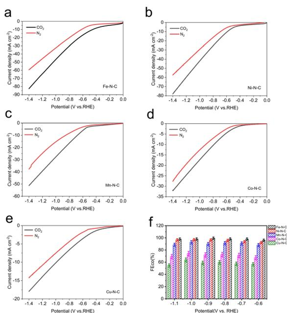
Fig. 4 Electrochemical performances for  $\text{CO}_2$  reduction. LSV curves of (a) Fe–N–C, (b) Ni–N–C, (c) Mn–N–C, (d) Co–N–C and (e) Cu–N–C in pure  $\text{N}_2$ - and  $\text{CO}_2$ -saturated  $0.5\text{ M KHCO}_3$  at a scan rate of  $10\text{ mV s}^{-1}$ . (f) The corresponding  $\text{FE}_{\text{CO}}$  at different applied potentials.
