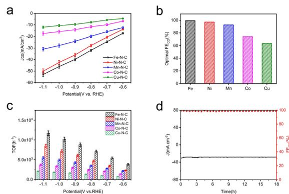
Fig. 5 Electrocatalytic  $\text{CO}_2$ RR performance of M–N–C catalysts in  $\text{CO}_2$ -saturated  $0.5\text{ M KHCO}_3$  electrolyte within a flow cell. (a)  $\text{CO}$  partial current density ( $J_{\text{CO}}$ ). (b) The optimal  $\text{FE}_{\text{CO}}$  and (c) TOFs at different applied potentials of all five catalysts. (d) Stability of Fe–N–C at  $-0.9\text{ V vs. RHE}$  for 18 h continuous electrolysis.
