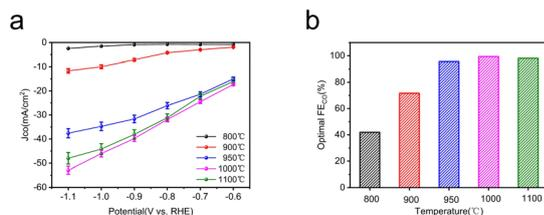
Fig. 7 Electrocatalytic CO<sub>2</sub>RR performance of Fe–N–C–T catalysts in CO<sub>2</sub>-saturated 0.5 M KHCO<sub>3</sub> electrolyte within a flow cell. (a) CO partial current density ( $J_{CO}$ ); (b) the optimal FE<sub>CO</sub>.
