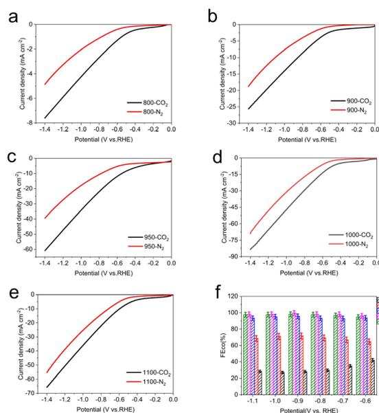
Fig. 6 Electrochemical performances for CO<sub>2</sub> reduction. LSV curves of Fe-N-C- $T$  (a) 800 °C, (b) 900 °C, (c) 950 °C, (d) 1000 °C and (e) 1100 °C in pure N<sub>2</sub>- and CO<sub>2</sub>-saturated 0.5 M KHCO<sub>3</sub> at a scan rate of 10 mV s<sup>-1</sup>. (f) The corresponding FE<sub>CO</sub> at different applied potentials.
