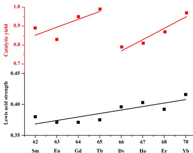
Fig. 4 The trend chart showing catalytic yield (activity) of Ln-MOFs vs. *Z*<sub>Ln</sub> in catalyzing CO<sub>2</sub>-cycloaddition reaction and the Lewis acid strength of Ln<sup>3+</sup> vs. *Z*<sub>Ln</sub>.
