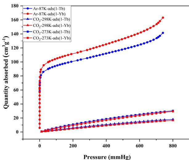
Fig. 3 The Ar adsorption isotherms at 87 K and the CO<sub>2</sub> adsorption isotherms at 273 K and 298 K of **1-Tb** and **1-Yb**.
