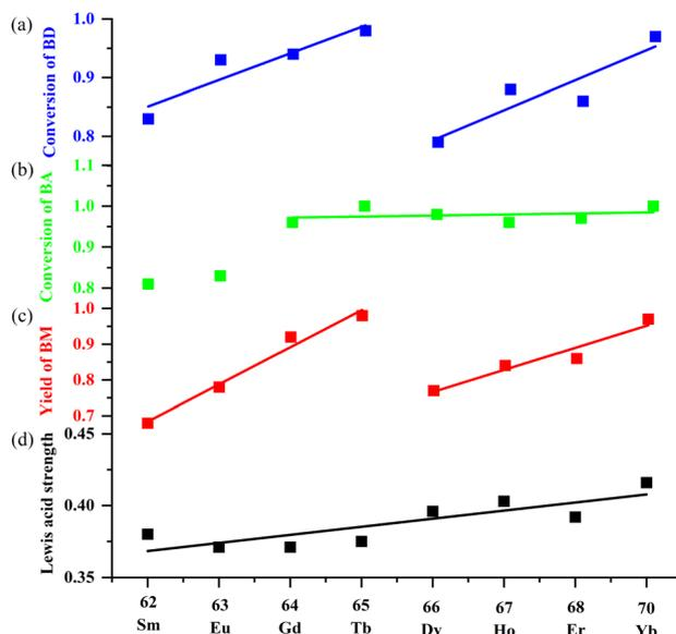
**Fig. 5** The trend chart showing (a) the conversion of BD, (b) the conversion of intermediate BA, and (c) the yield of BM vs.  $Z_{Ln}$  (the coordination number of Ln) in catalyzing one-pot cascade reaction and (d) the Lewis acid strength of Ln<sup>3+</sup> vs.  $Z_{Ln}$ .
