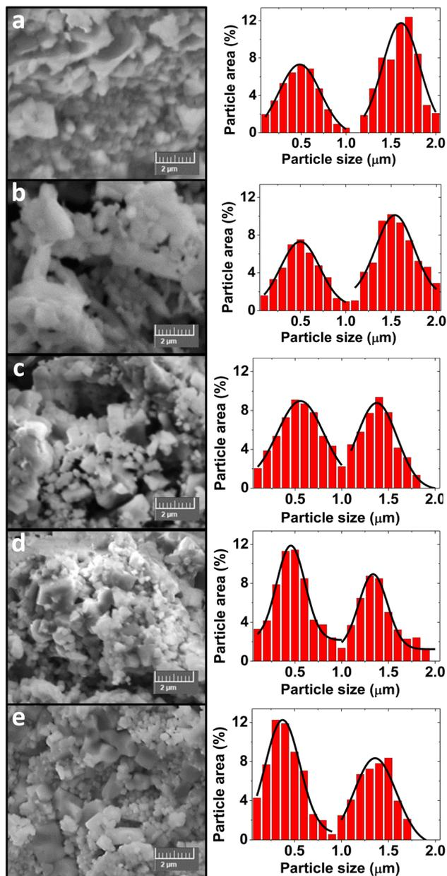
Fig. 3 SEM images (left column) and particle size distributions (right column) of the  $\text{CFO}_x/\text{NCZO}_y$  composites. (a)  $\text{CFO}_3/\text{NCZO}_1$ . (b)  $\text{CFO}_2/\text{NCZO}_1$ . (c)  $\text{CFO}_1/\text{NCZO}_1$ . (d)  $\text{CFO}_1/\text{NCZO}_2$ . (e)  $\text{CFO}_1/\text{NCZO}_3$ .
