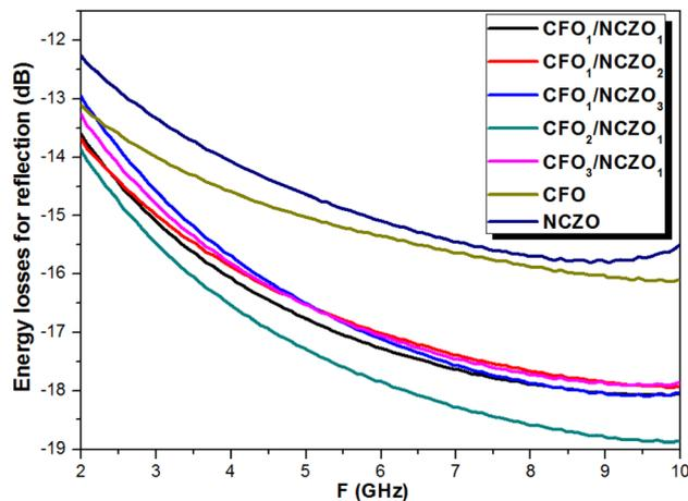
Fig. 9 Energy losses behavior vs. frequency for the CFO<sub>x</sub>/NCZO<sub>y</sub> composites in the range 2–10 GHz.
