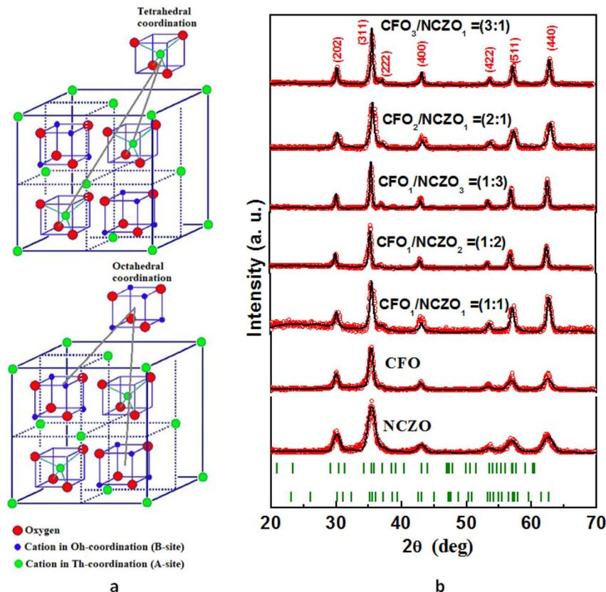
Fig. 1 Features of the crystal structure of the  $\text{CFO}_x/\text{NCZO}_y$  composites. (a) Crystal structure of the spinel-like ferrite with SG:  $Fd\bar{3}m$ . (b) XRD patterns of the  $\text{CFO}_x/\text{NCZO}_y$  composites.
