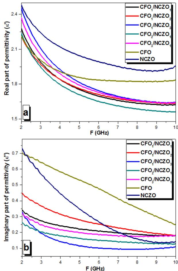
Fig. 7 Permittivity behavior vs. frequency for the  $\text{CFO}_x/\text{NCZO}_y$  composites in the range 2–10 GHz. (a) Real part of the permittivity –  $\epsilon'$ . (b) Imaginary part of the permittivity –  $\epsilon''$ .
