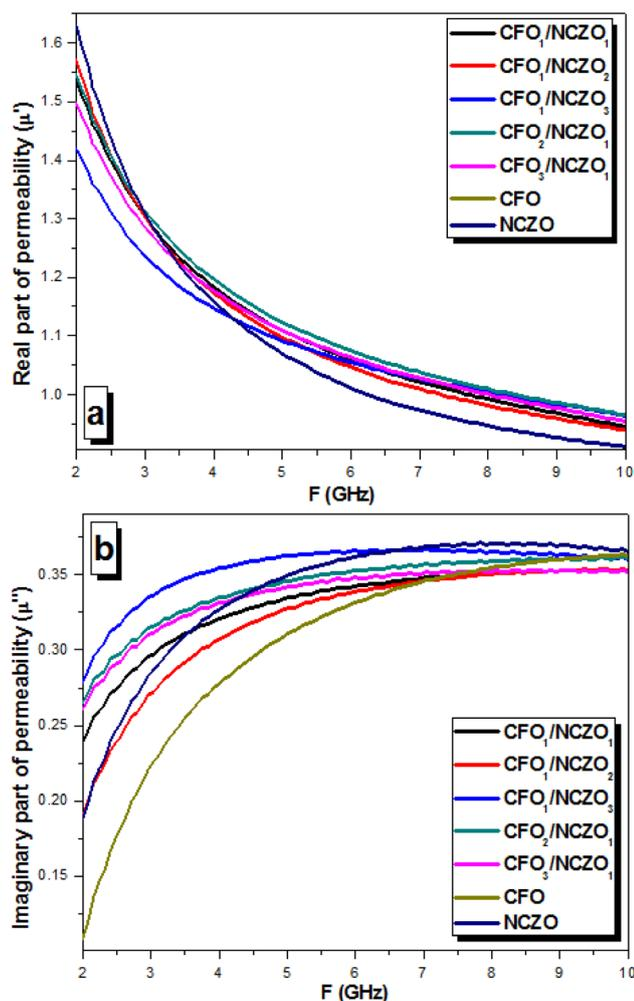
Fig. 8 Permeability behavior vs. frequency for the CFO<sub>x</sub>/NCZO<sub>y</sub> composites in the range 2–10 GHz. (a) Real part of the permeability –  $\mu'$ . (b) Imaginary part of the permeability –  $\mu''$ .
