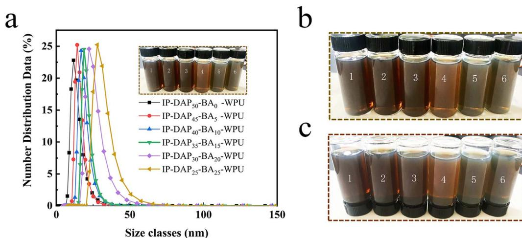
Fig. 1 (a) Particle size and distribution of the as-prepared WPU particles. Color and appearance of IP-DAP<sub>x</sub>-BA<sub>y</sub>-WPU emulsions (b) before and (c) after centrifugation in natural light.
