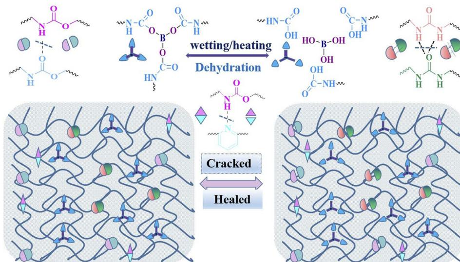
Fig. 9 Schematic diagram of self-healable mechanism of IP-DAP<sub>x</sub>-BA<sub>y</sub>-WPU film.
