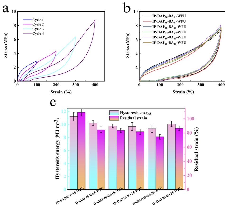
Fig. 5 (a) Sequential cyclic tensile curves of the IP-DAP<sub>30</sub>-BA<sub>20</sub>-WPU film at different strains without waiting time. (b) Cyclic tensile curves of IP-DAP<sub>x</sub>-BA<sub>y</sub>-WPU films with a maximum strain of 400%. (c) Residual strain and hysteresis energy of IP-DAP<sub>x</sub>-BA<sub>y</sub>-WPU films during the cyclic tensile processes.
