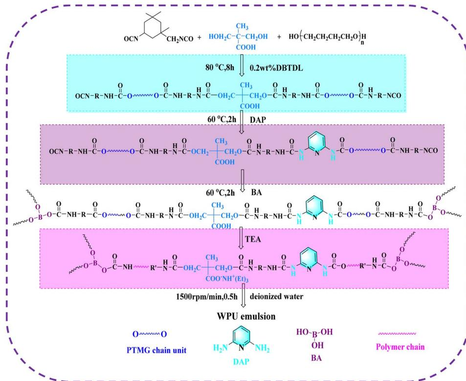
Scheme 1 Synthetic route for IP-DAP<sub>x</sub>-BA<sub>y</sub>-WPU emulsion.Table 1 Composition of reactants for the synthesis of IP-DAP<sub>x</sub>-BA<sub>y</sub>-WPU (mmol)
