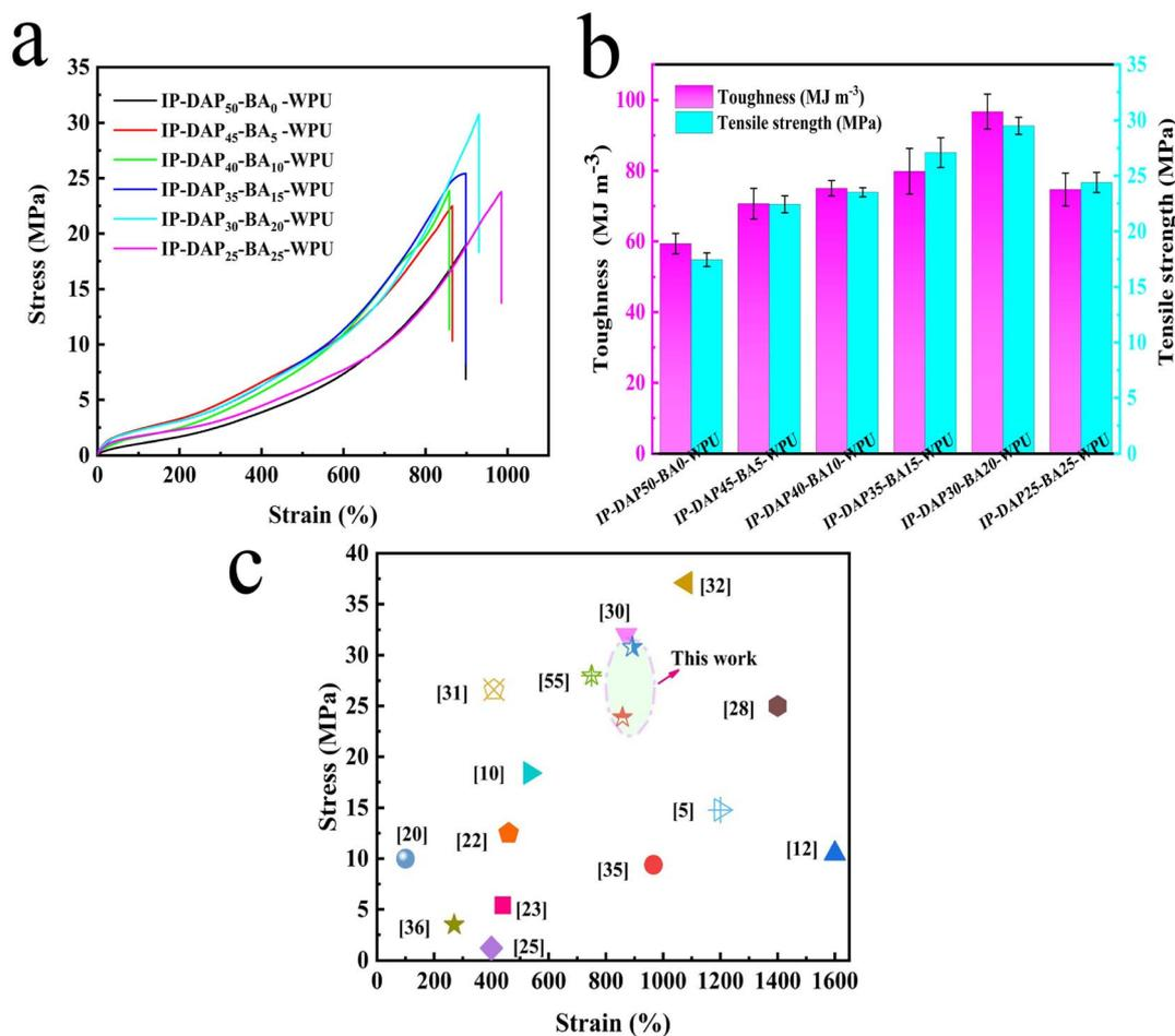
Fig. 4 (a) Stress–strain curves. (b) Tensile strength and toughness of different IP-DAP<sub>x</sub>-BA<sub>y</sub>-WPU films. (c) Mechanical performance of the representative IP-DAP<sub>40</sub>-BA<sub>10</sub>-WPU and IP-DAP<sub>30</sub>-BA<sub>20</sub>-WPU films in this work compared with those of other studies.
