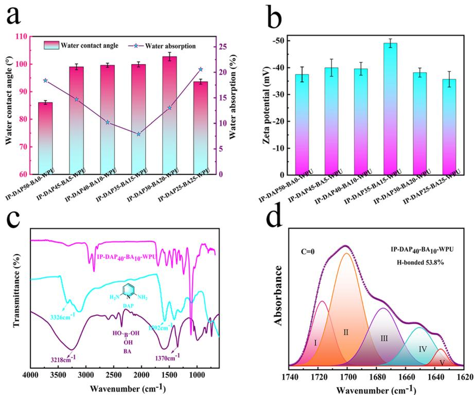
Fig. 2 (a) Water contact angle (WCA) and water absorption (WA) of different IP-DAP<sub>x</sub>-BA<sub>y</sub>-WPU samples. (b) Zeta potential values of different IP-DAP<sub>x</sub>-BA<sub>y</sub>-WPU emulsions. (c) FT-IR spectra of BA, DAP and IP-DAP<sub>40</sub>-BA<sub>10</sub>-WPU in the frequency range of 650–4000 cm<sup>-1</sup>. (d) FTIR spectra of IP-DAP<sub>40</sub>-BA<sub>10</sub>-WPU in the C=O stretching vibration region.
