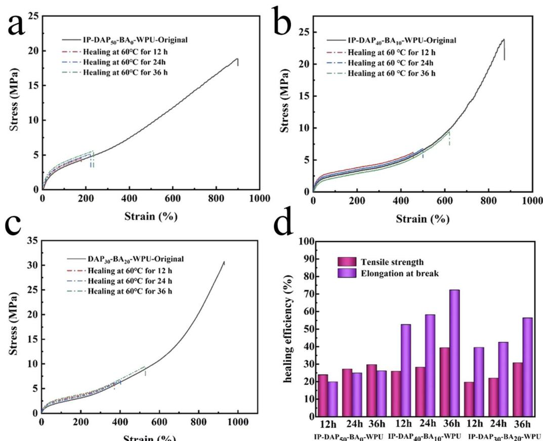
Fig. 6 Original and self-healed tensile stress–strain curves (a–c) and self-healing efficiency (d) of IP-DAP<sub>50</sub>-BA<sub>0</sub>-WPU, IP-DAP<sub>40</sub>-BA<sub>10</sub>-WPU and IP-DAP<sub>30</sub>-BA<sub>20</sub>-WPU films after healing at 60 °C for 12 h, 24 h, and 36 h.
