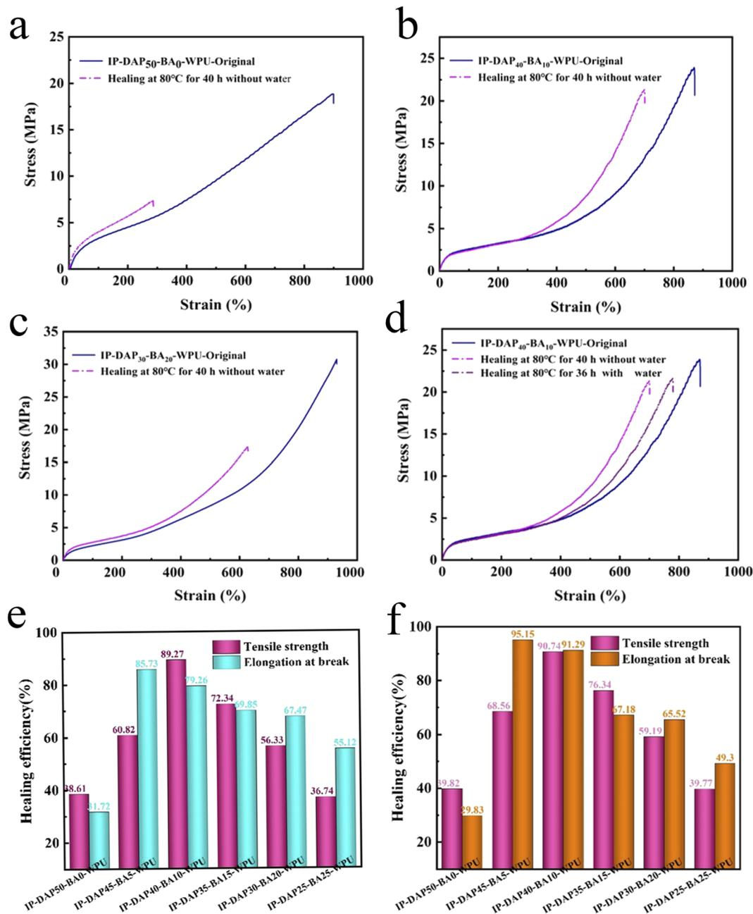
Fig. 7 Original and self-healed tensile stress–strain curves (a–c) of IP-DAP<sub>x</sub>-BA<sub>y</sub>-WPU films after heating at 80 °C for 40 h without water. (d) Representative original and self-healed tensile stress–strain curves of IP-DAP<sub>40</sub>-BA<sub>10</sub>-WPU films under different conditions. (e) Self-healing efficiency of IP-DAP<sub>x</sub>-BA<sub>y</sub>-WPU films heated at 80 °C for 40 h without water and (f) heated at 80 °C for 36 h with the aid of water.
