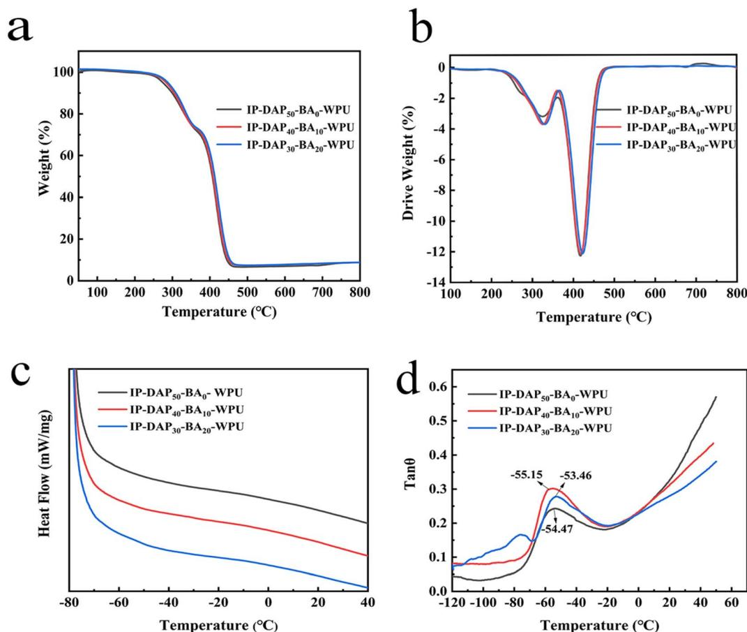
Fig. 3 (a) TGA curves, (b) DTG curves, (c) DSC curves, and (d) loss factor ( $\tan \theta$ ) of the representative IP-DAP<sub>50</sub>-BA<sub>0</sub>-WPU, IP-DAP<sub>40</sub>-BA<sub>10</sub>-WPU and IP-DAP<sub>30</sub>-BA<sub>20</sub>-WPU samples.
