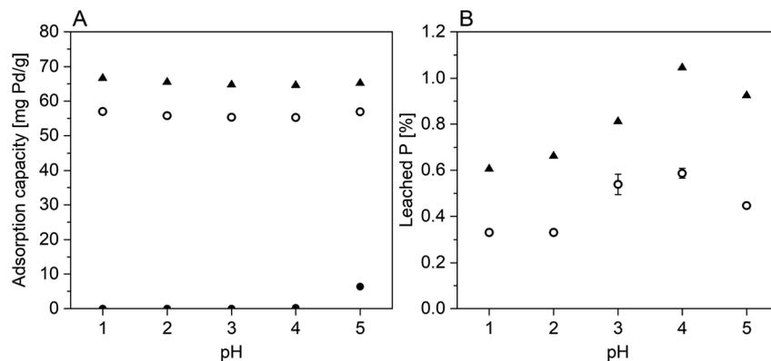
Fig. 4 Effect of pH on the adsorption capacity of Pd ( $\text{mg g}^{-1}$ , A) and the relative amount of leached phosphorus (%), B) between pH 1 and 5 for native Hombikat M311 (closed circles), 3MPPA50 (open circles) and 3MPPA150 (triangles). Adsorbent dose =  $2.5 \text{ g L}^{-1}$ ,  $t = 24 \text{ h}$ ,  $C_{\text{Pd}} = 250 \text{ mg L}^{-1}$ ,  $0.1 \text{ M Cl}^{-}$ .
