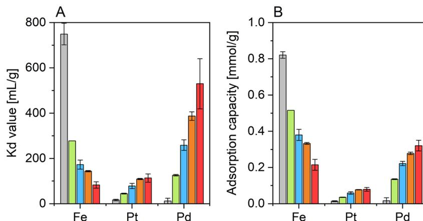
**Fig. 8** (A) Distribution coefficient values ( $K_d$ ) and (B) adsorption capacity ( $\text{mmol g}^{-1}$ ) for Fe, Pd and Pt in the automotive catalyst acidic leachate upon adsorption on native Hombikat M311 (grey) and 3MPPA grafted Hombikat M311 with different surface coverages. 3MPPA20 (green), 3MPPA50 (blue), 3MPPA100 (orange) and 3MPPA150 (red).
