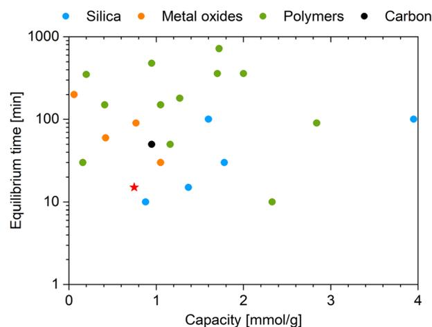
Fig. 9 Plot of the maximal palladium adsorption capacity (mmol g<sup>-1</sup>) and equilibrium time (min) for different classes of sulfur-containing adsorbents (silica materials, metal oxides, (bio)polymers and carbon-based). The plotted data points are based on the adsorption capacities and equilibrium times depicted in Table 6. The red star represents 3MPPA150 (this study).
