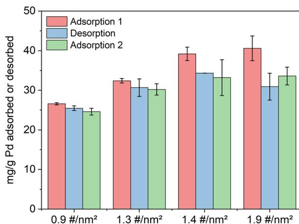
Fig. 7 Pd adsorption, recovery and adsorption capacity ( $\text{mg g}^{-1}$ ) in consecutive steps. Adsorbent dose =  $2.5 \text{ g L}^{-1}$ ,  $\text{pH} = 2.0$ ,  $t = 30 \text{ min}$ ,  $C_{\text{Pd}} = 250 \text{ mg L}^{-1}$ .
